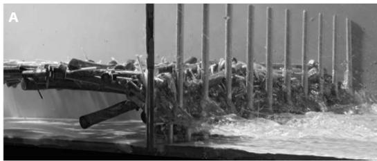
**Figure 2.8:** Wooden debris accumulation (curved blockage) [36]
