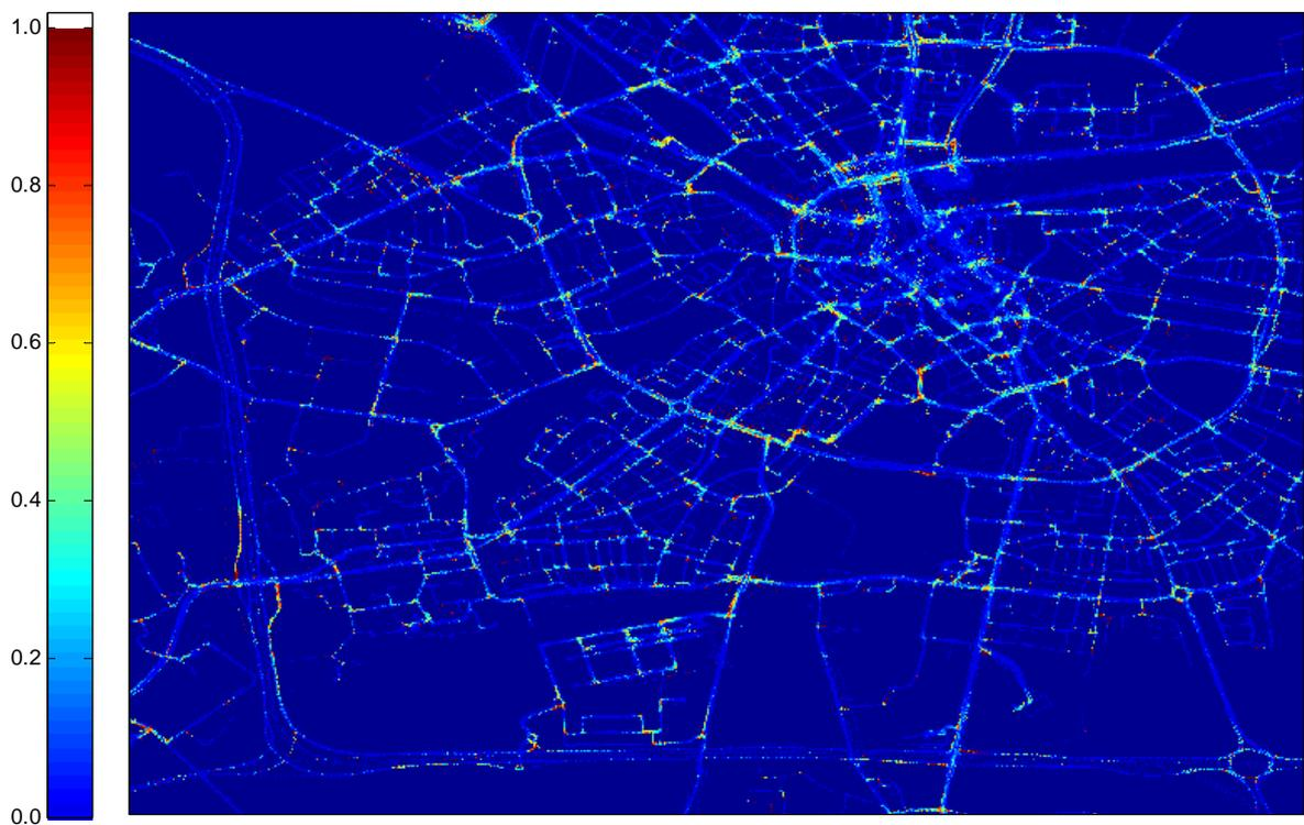
Figure 58: Direction indicator usage in Eindhoven. The color scale represents which part of the uCAN equipped vehicles uses its direction indicators while being at a specific location. Dark blue (the background color) indicates that no vehicles
