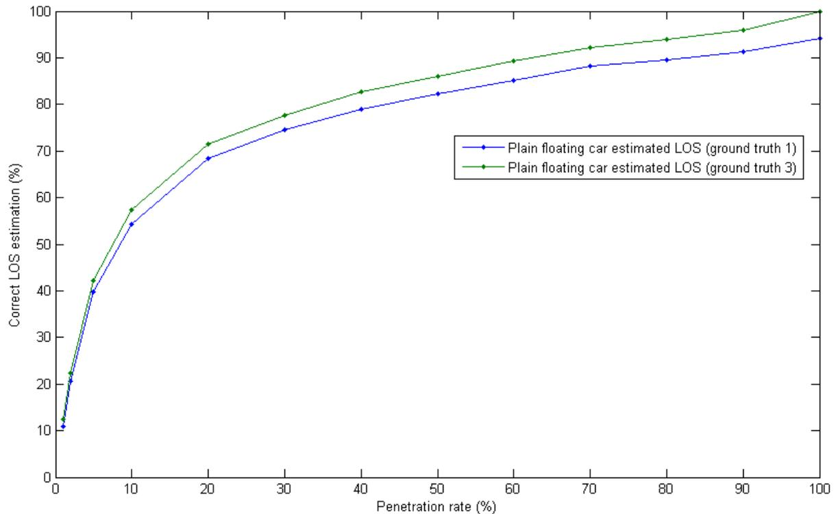
Figure 30: Penetration rate versus correct LOS estimation with simulated plain floating car data (containing only positional data), for ground truth 1, determined with simulation loop detector data, and ground truth 3, determined with the vehicle presence, for all minutes.
