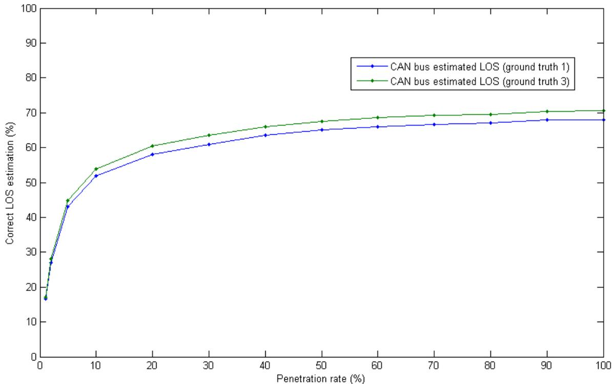
Figure 28: Penetration rate versus correct LOS estimation with simulated average CAN bus speed, for ground truth 1, determined with simulation loop detector data, and ground truth 3, determined with the vehicle presence, for all minutes.
