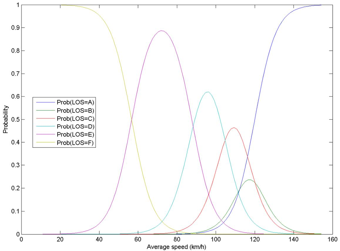
Figure 77: LOS probability functions for 10% penetration
