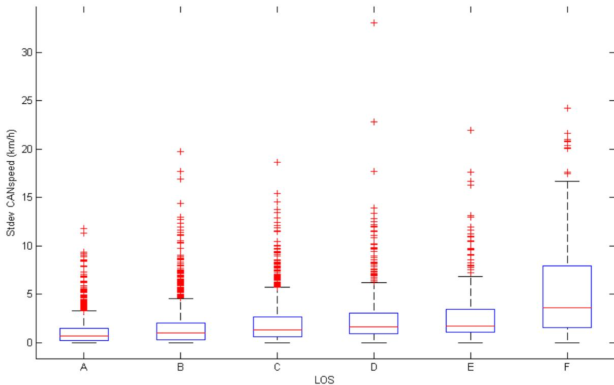
Figure 14: LOS versus st.dev. of CAN bus speed. The standard deviation of the CAN bus speed of the uCAN equipped vehicles passing a loop detector is plotted against the Level of Service ground truth in the corresponding minute.
