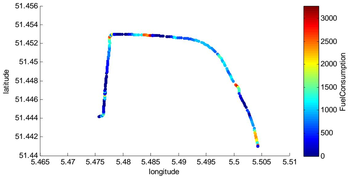
Figure 49: Position and fuel consumption during the trip. The color scale indicates the fuel consumption of the vehicle. The unit of the fuel consumption is unknown.
