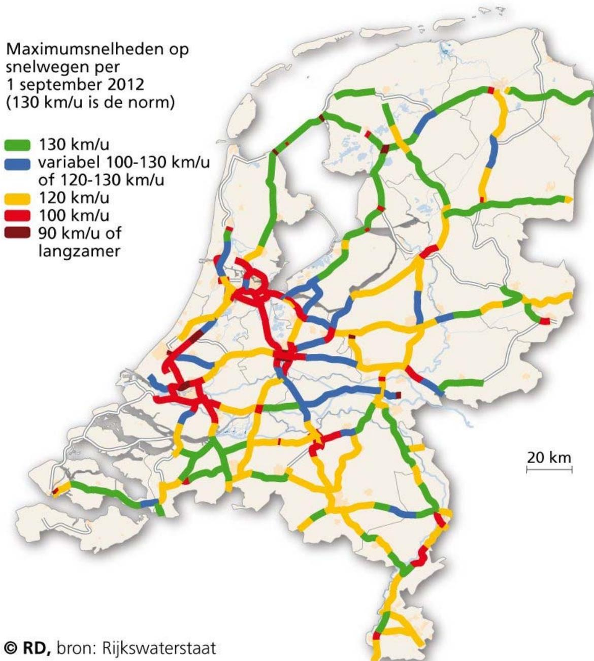
Figure 69: Speed limits on Dutch motorways [47]
