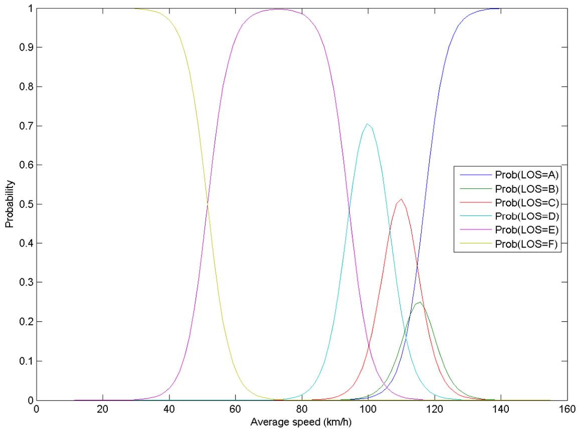
Figure 81: LOS probability functions for 50% penetration
