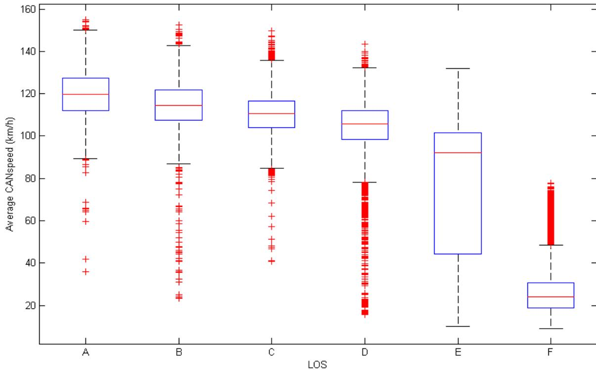
Figure 22: LOS ground truth 1 versus average speed. The average simulated CAN bus speed of the simulated vehicles passing a detection point is plotted against the Level of Service ground truth in the corresponding minute, determined with the detection point data.
