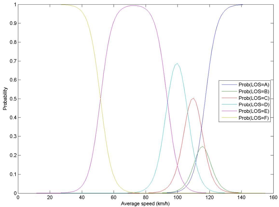
Figure 79: LOS probability functions for 30% penetration
