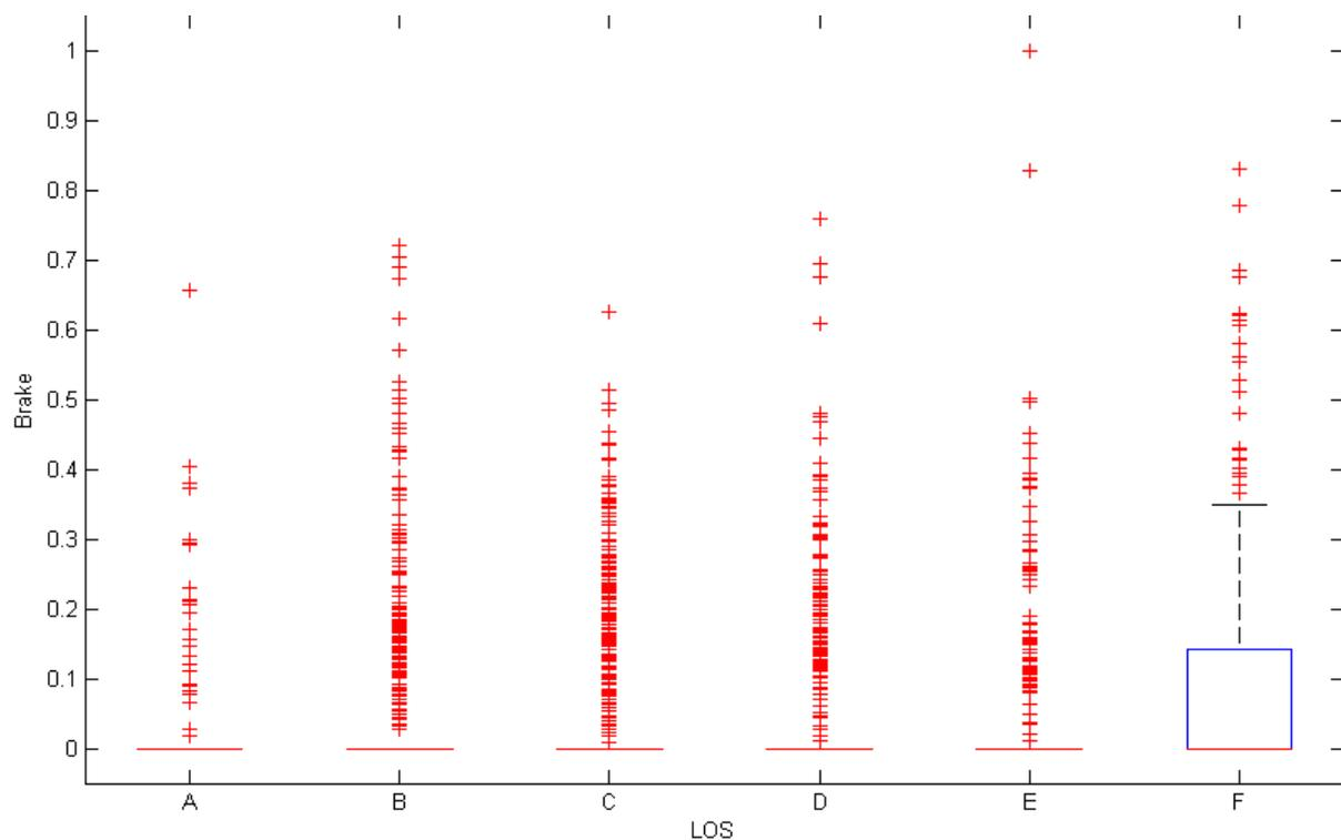
Figure 18: LOS versus average brake usage. The average brake usage (the number of seconds in which the brake was used during the vehicle passage divided by the total number of seconds of the vehicle passage) of the uCAN equipped vehicles passing a loop detector is plotted against the Level of Service ground truth in the corresponding minute.
