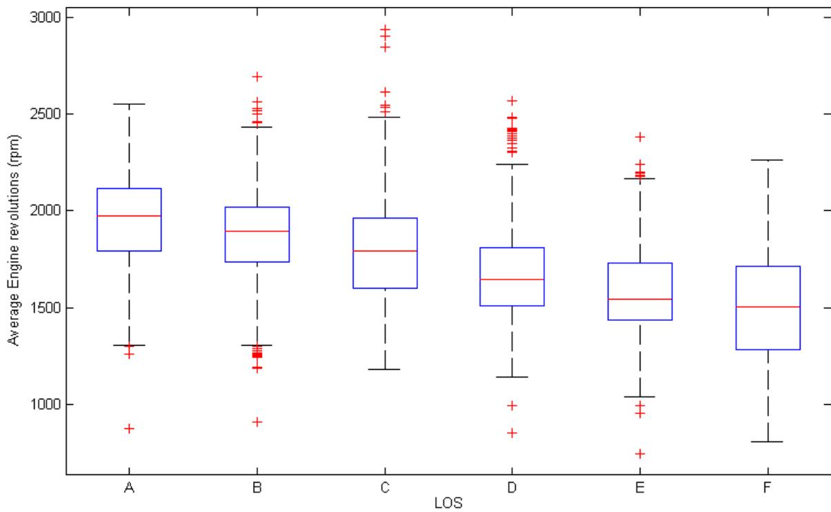
Figure 19: LOS versus average engine rotational speed. The average engine rotational speed of the uCAN equipped vehicles passing a loop detector is plotted against the Level of Service ground truth in the corresponding minute.
