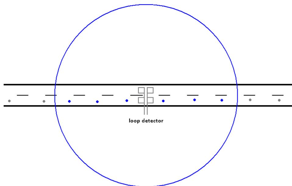
Figure 7: Combining the CAN bus data with the loop detector data. The dots indicate the GPS coordinates of the data points of a uCAN equipped vehicle. The blue circle, determined by the loop detector position and the radius, indicates the area in which the CAN bus data points are collected.
