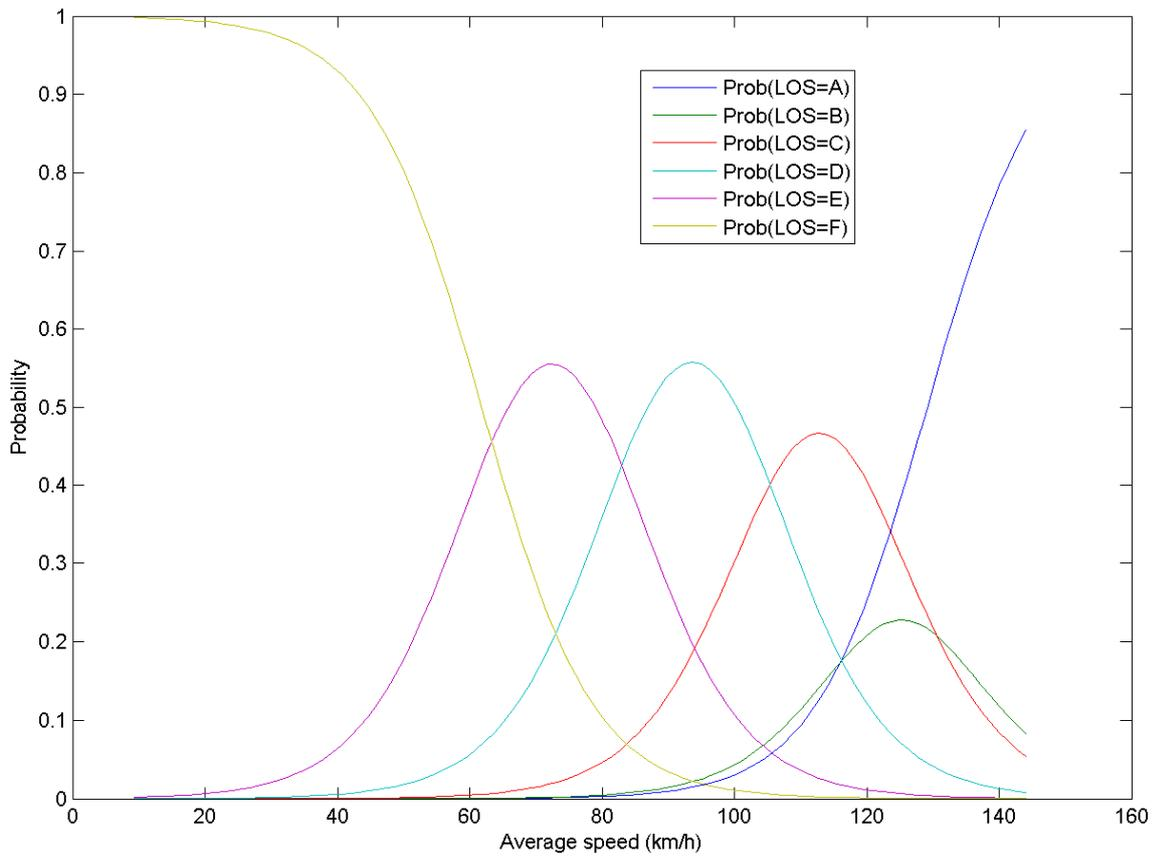
Figure 75: LOS probability functions for 2% penetration
