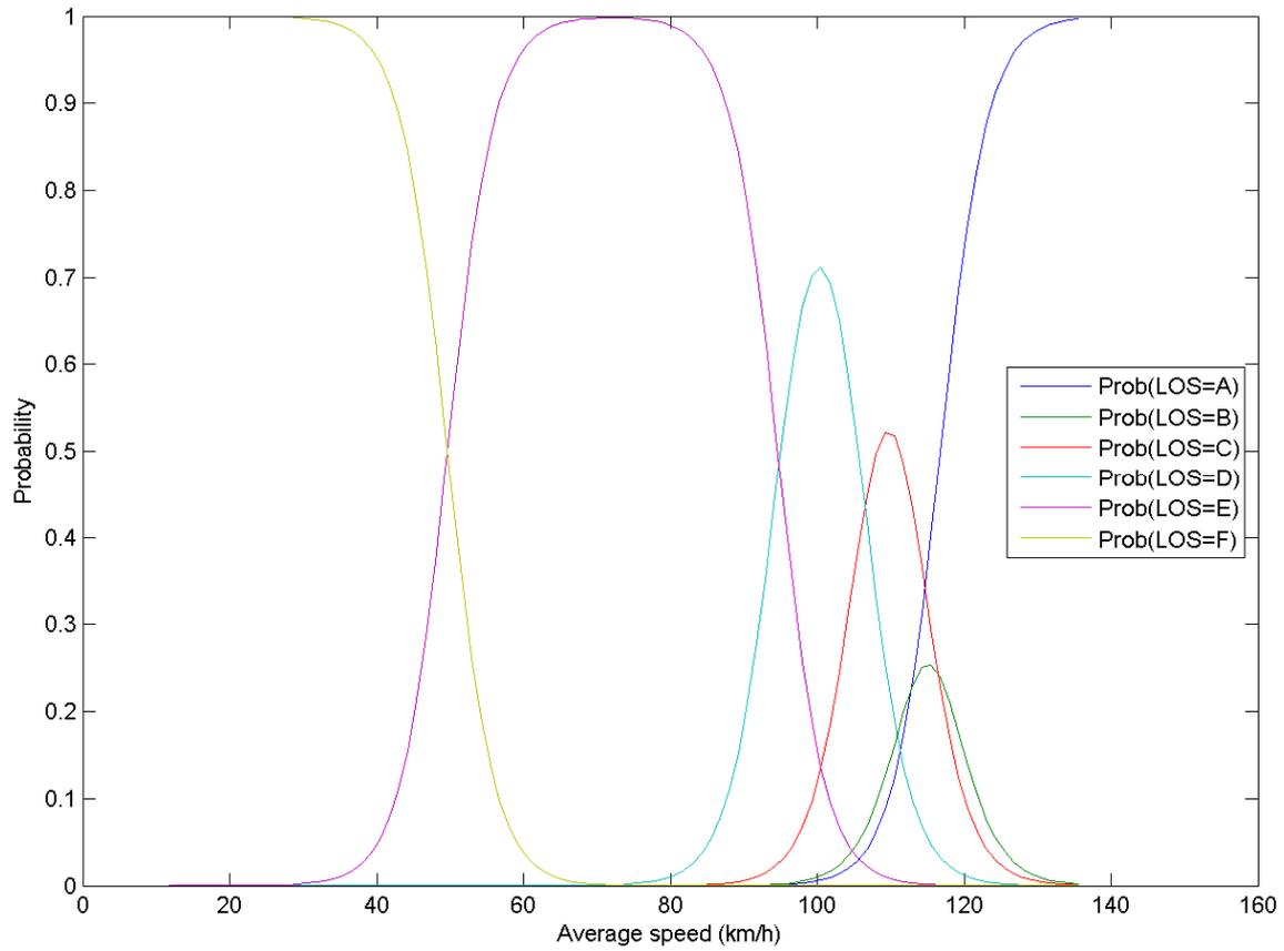
Figure 82: LOS probability functions for 60% penetration
