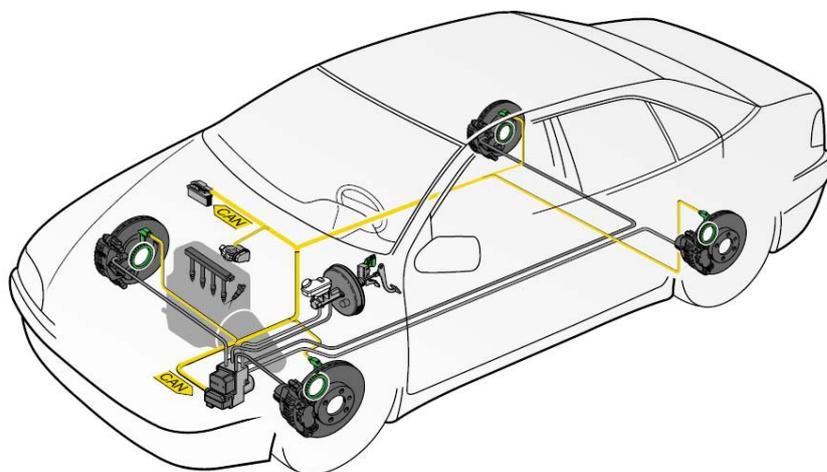
Figure 1: Traction control CAN bus [4]
