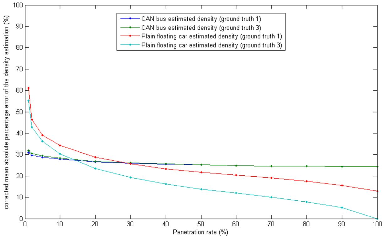
Figure 33: Corrected Mean Absolute Percentage Error of the density estimation with simulated CAN bus data and simulated plain floating car data (only containing positional data) using multiple vehicles, for different penetration rates. The 1-minute aggregated density ground truth is determined with the simulated detection point data (ground truth 1) and with the real density near the detection point, using the simulated vehicle trajectories (ground truth 3).
