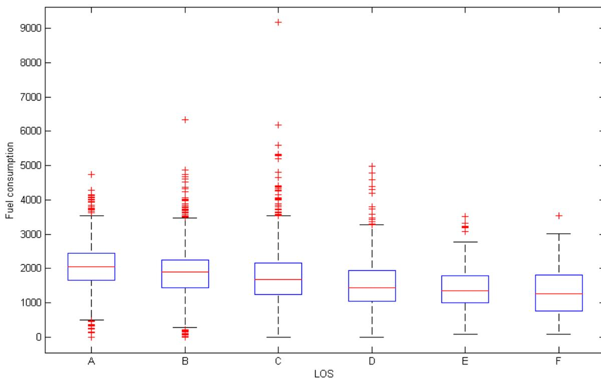
Figure 15: LOS versus average fuel consumption. The average fuel consumption of the uCAN equipped vehicles passing a loop detector is plotted against the Level of Service ground truth in the corresponding minute. The unit of fuel consumption is unknown.
