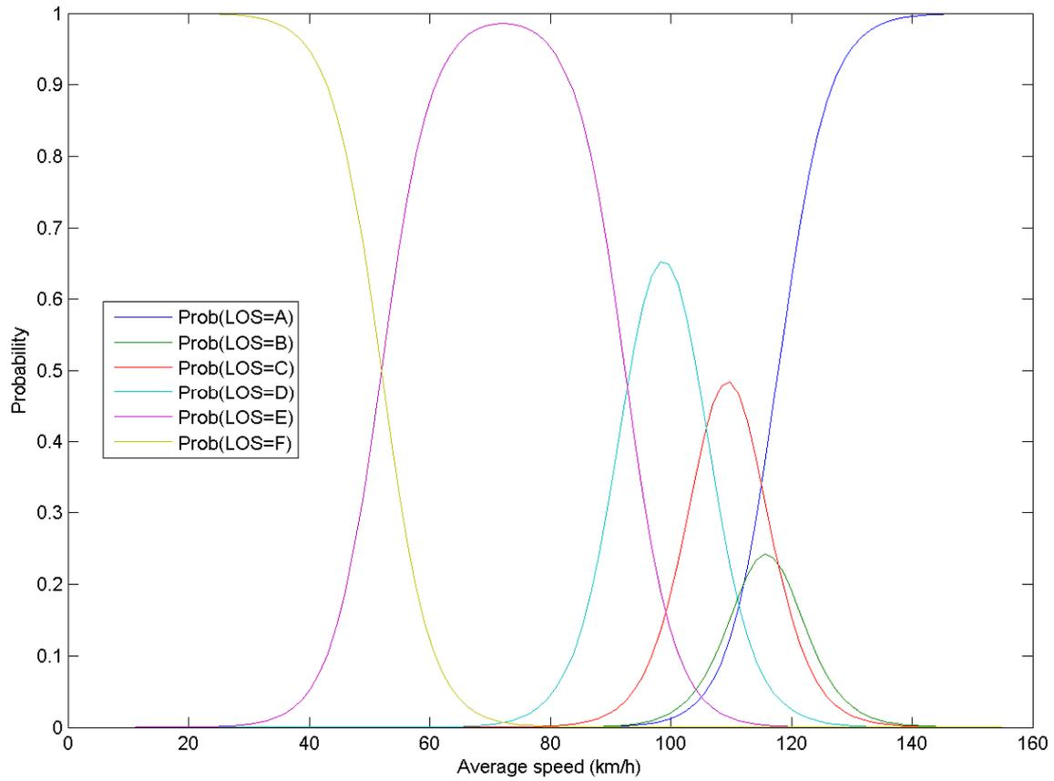
Figure 78: LOS probability functions for 20% penetration
