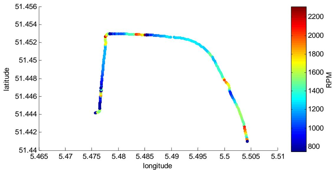
Figure 48: Position and RPM during the trip. The color scale indicates the engine revolution per minute.
