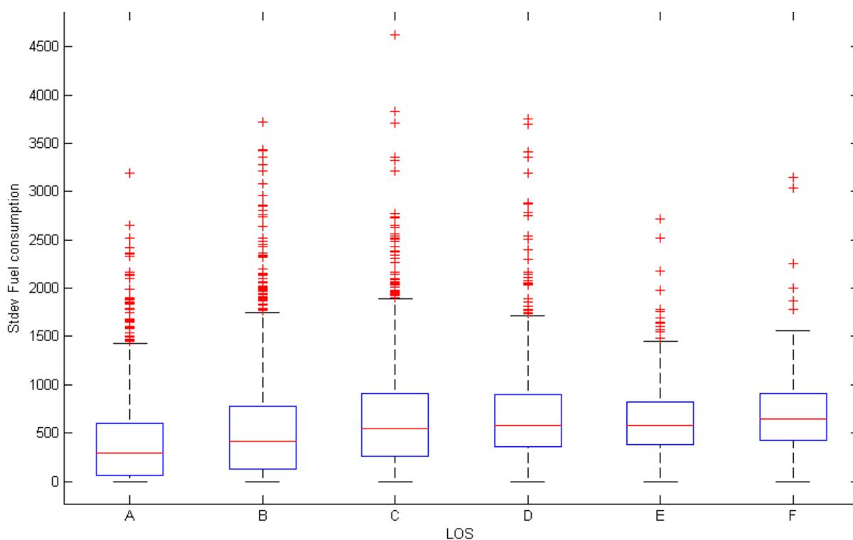
Figure 16: LOS versus st.dev of fuel consumption. The standard deviation of fuel consumption of the uCAN equipped vehicles passing a loop detector is plotted against the Level of Service ground truth in the corresponding minute. The unit of fuel consumption is unknown.
