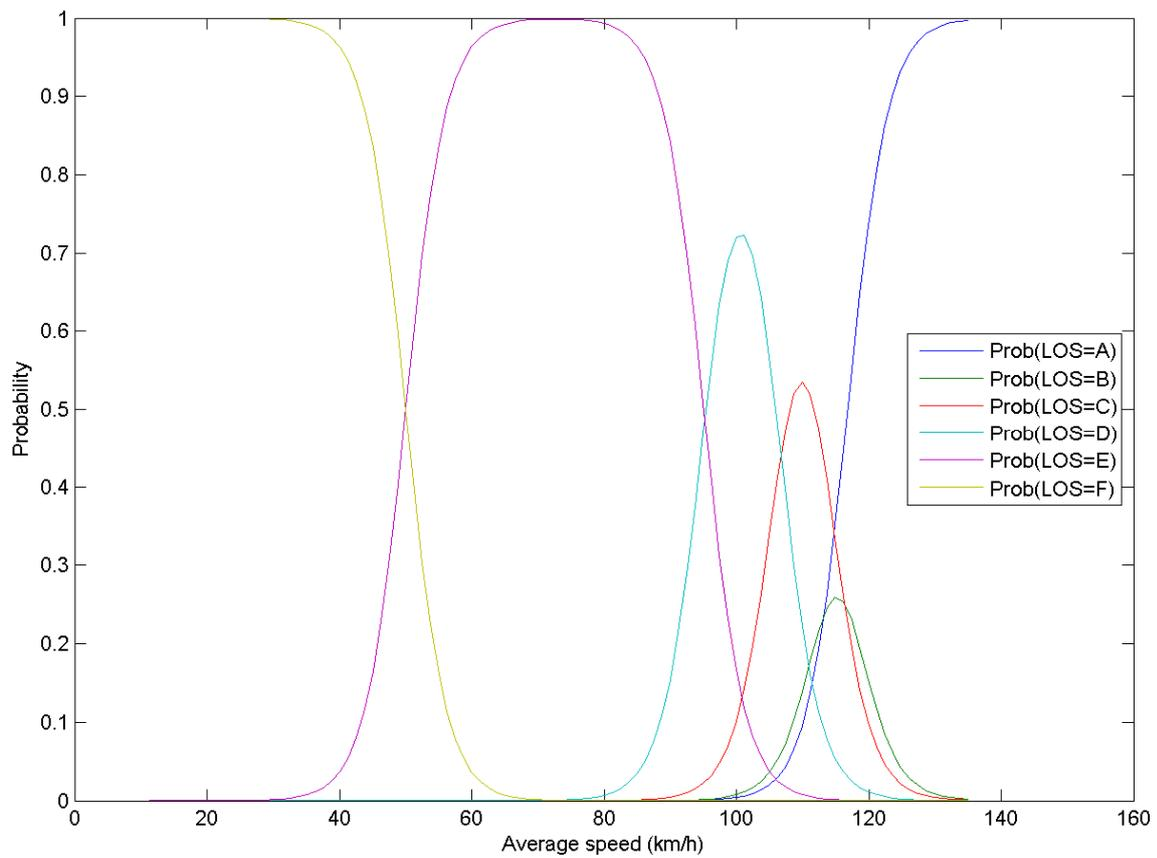
Figure 85: LOS probability functions for 90% penetration
