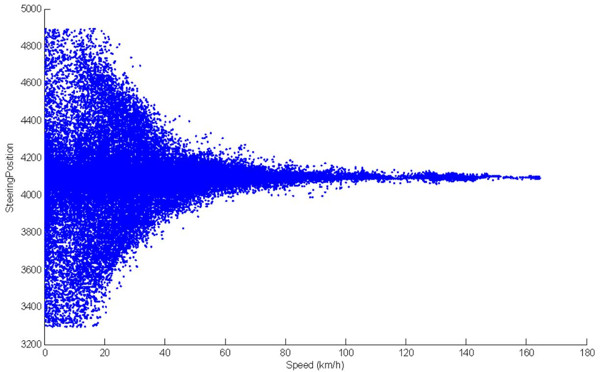
Figure 52: Speed versus steering position. The unit of the steering position is unknown.
