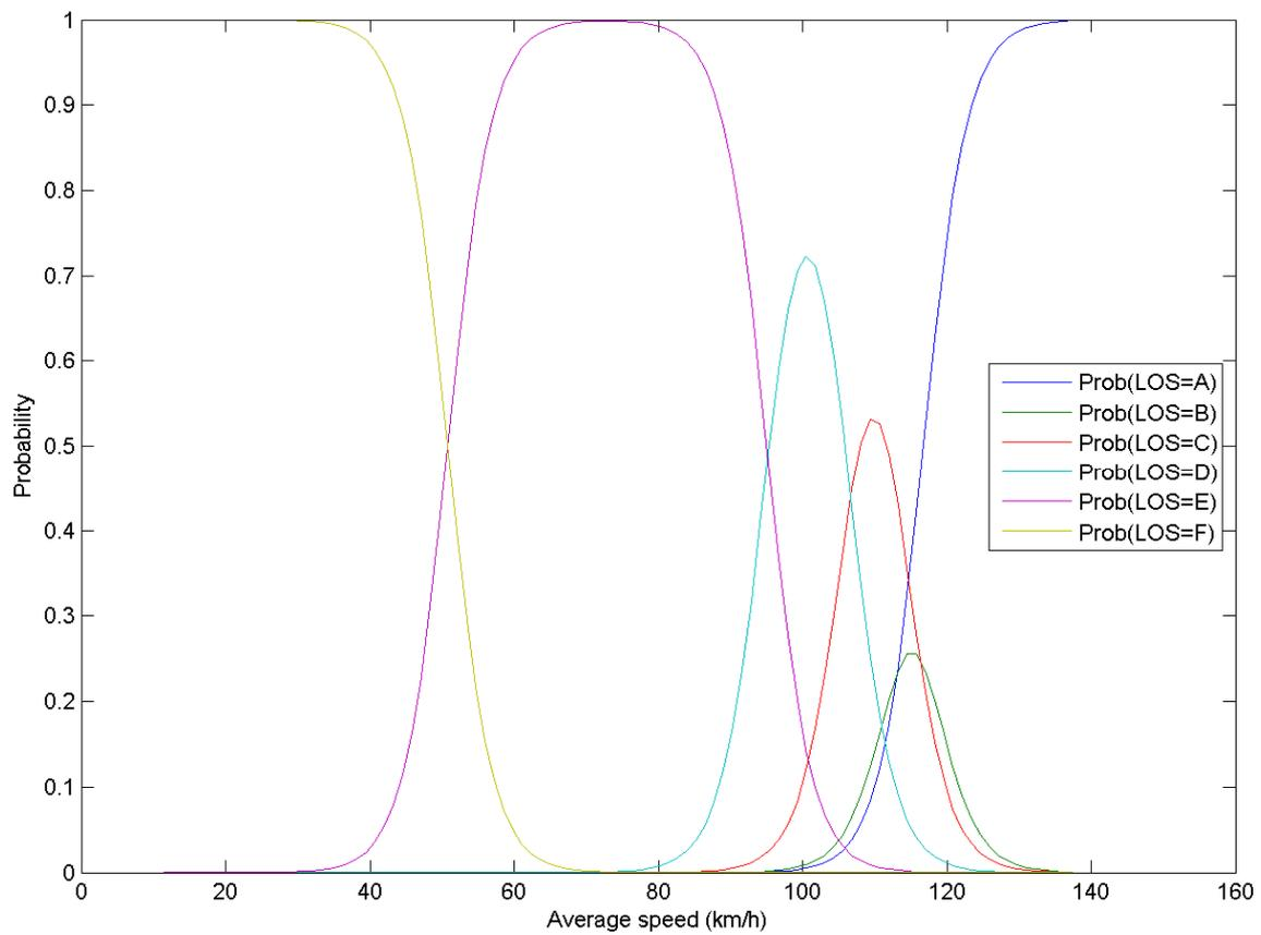
Figure 83: LOS probability functions for 70% penetration
