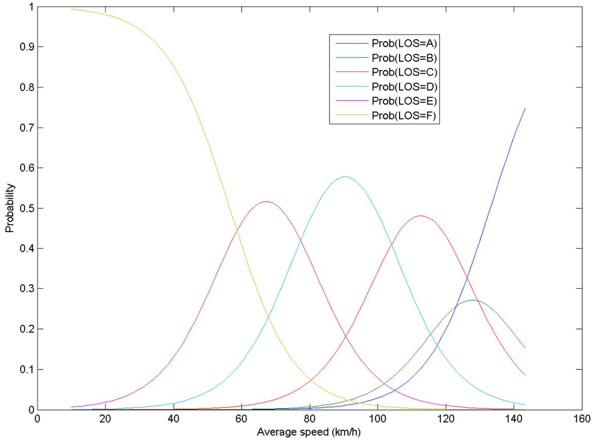
Figure 74: LOS probability functions for 1% penetration
