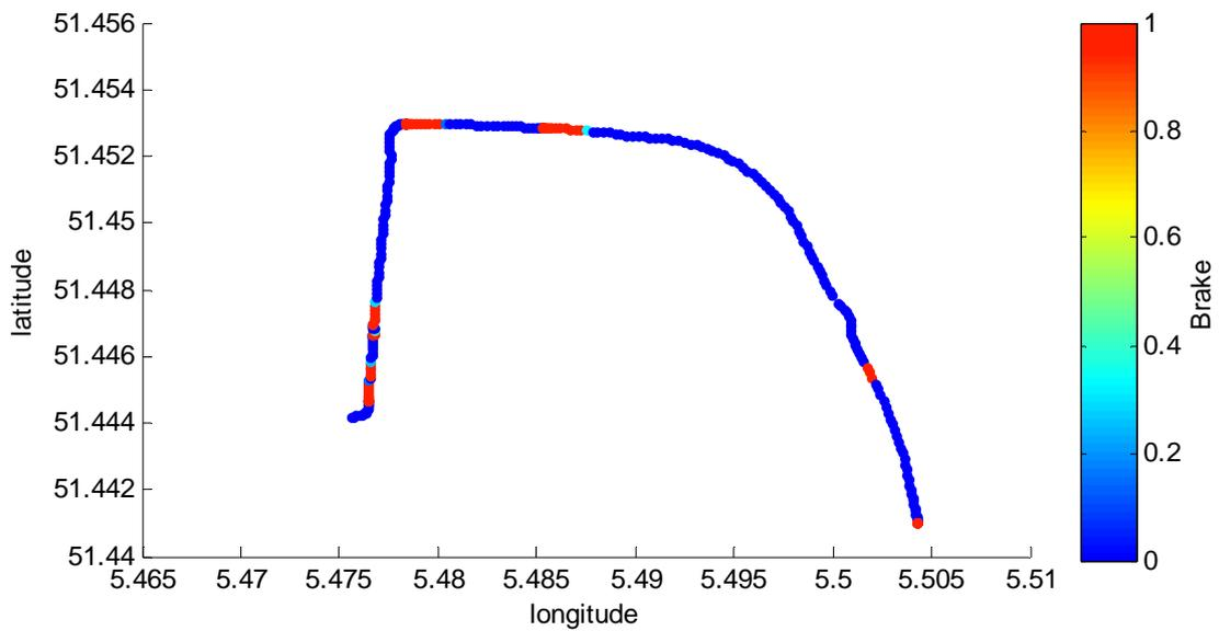
Figure 50: Position and brake usage during the trip. Red indicates the usage of the brakes. Blue indicates the brakes were not used.
