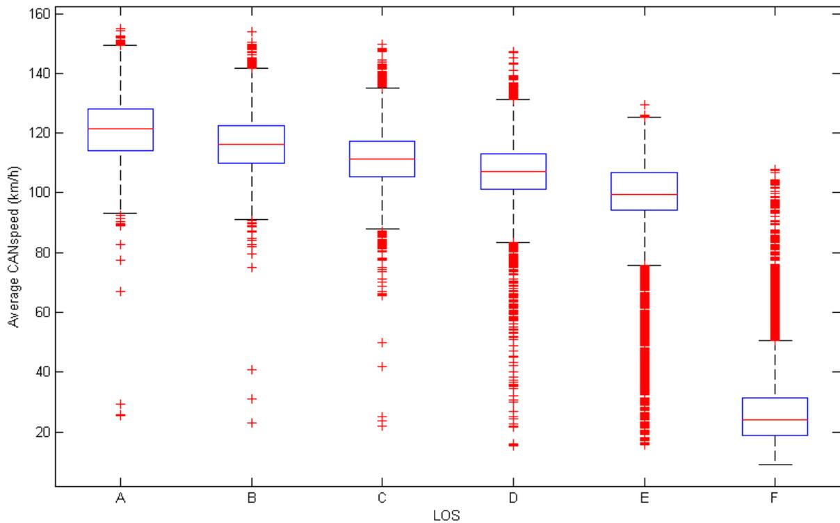
Figure 24: LOS ground truth 3 versus average speed. The average simulated CAN bus speed of the simulated vehicles passing a detection point is plotted against the Level of Service ground truth in the corresponding minute, determined with the presence of the simulated vehicles near the detection point.
