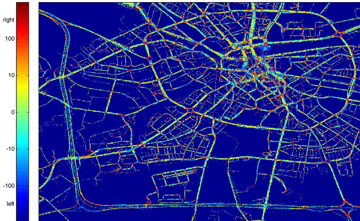
Figure 59: Steering position in Eindhoven. The color scale represents the average steering position of the uCAN equipped vehicles while being at a specific location. Dark blue (the background color) indicates that no vehicles in the data set have been at that location. Blue indicates that the vehicles on average are making a left turn at the location. Red indicates that the vehicles on average are making a right turn at the location.
