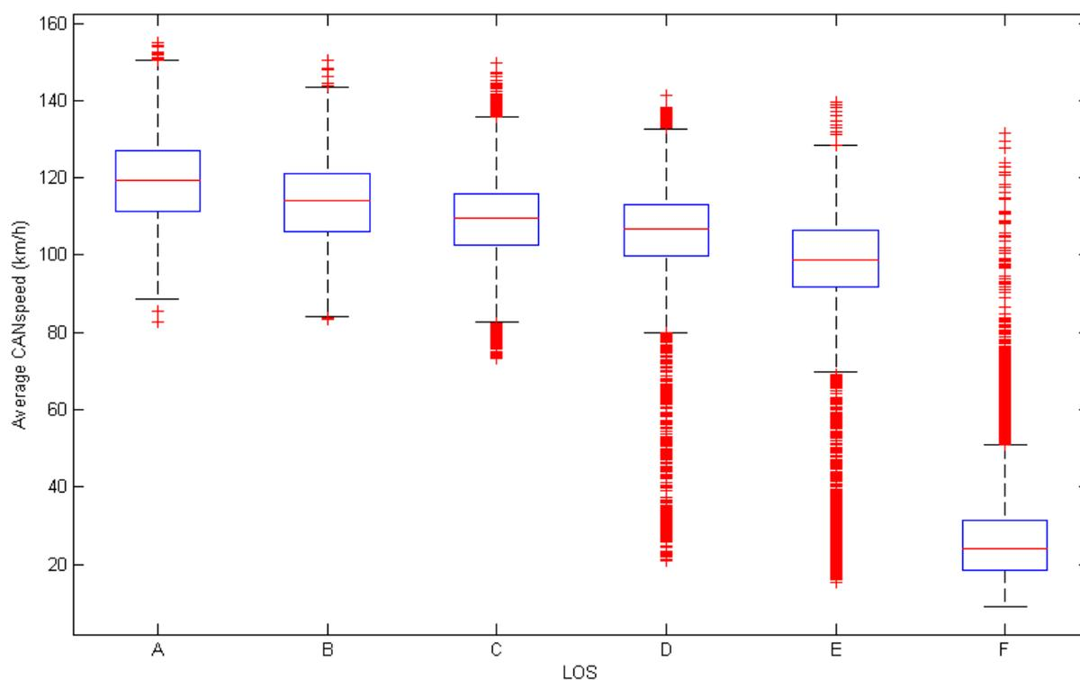
Figure 25: LOS ground truth 4 versus average speed. The average simulated CAN bus speed of the simulated vehicles passing a detection point is plotted against the Level of Service ground truth at that moment, determined with the presence of the simulated vehicles near the detection point.
