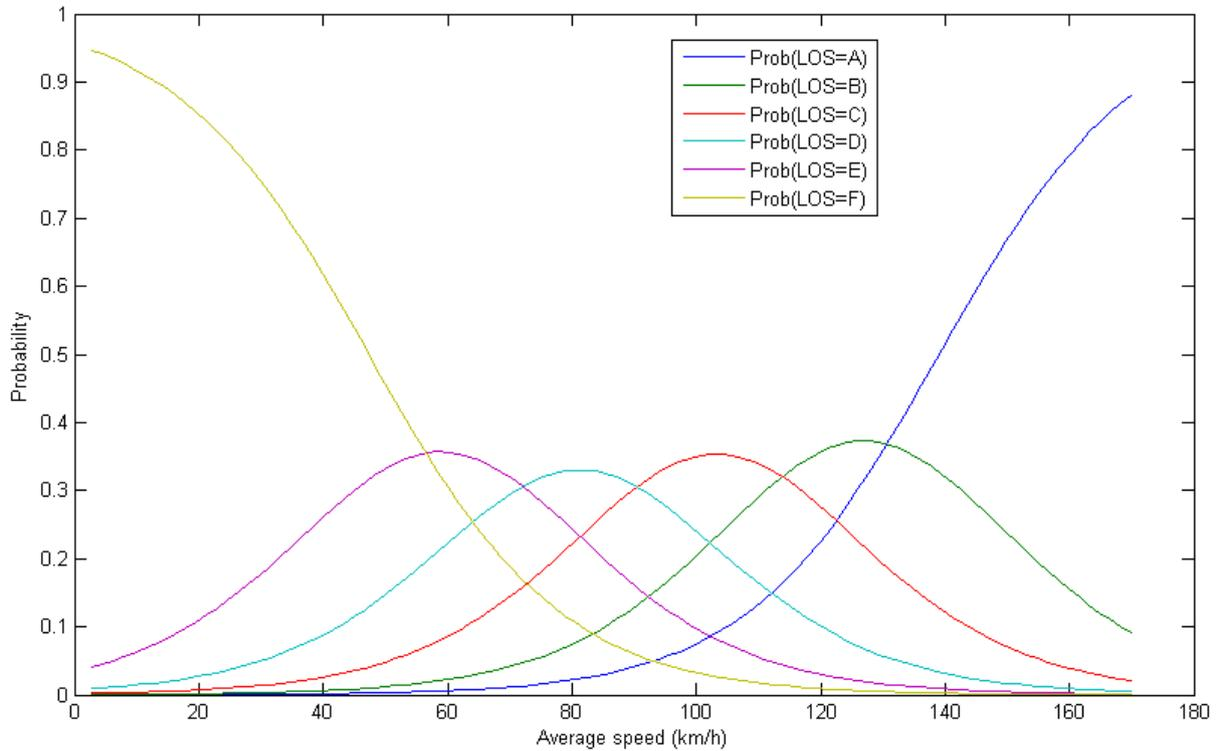
**Figure 21: LOS probability functions.** The functions indicate, for every value of the average speed of the passing uCAN equipped vehicle, the probability of occurrence of every LOS. The LOS with the highest probability is selected as LOS estimation.
