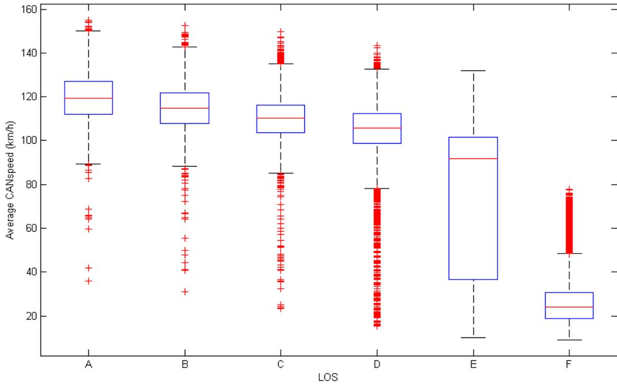
Figure 23: LOS ground truth 2 versus average speed. The average simulated CAN bus speed of the simulated vehicles passing a detection point is plotted against the Level of Service ground truth in the corresponding minute, determined with the detection point data, including an error, simulating real loop detector performance.
