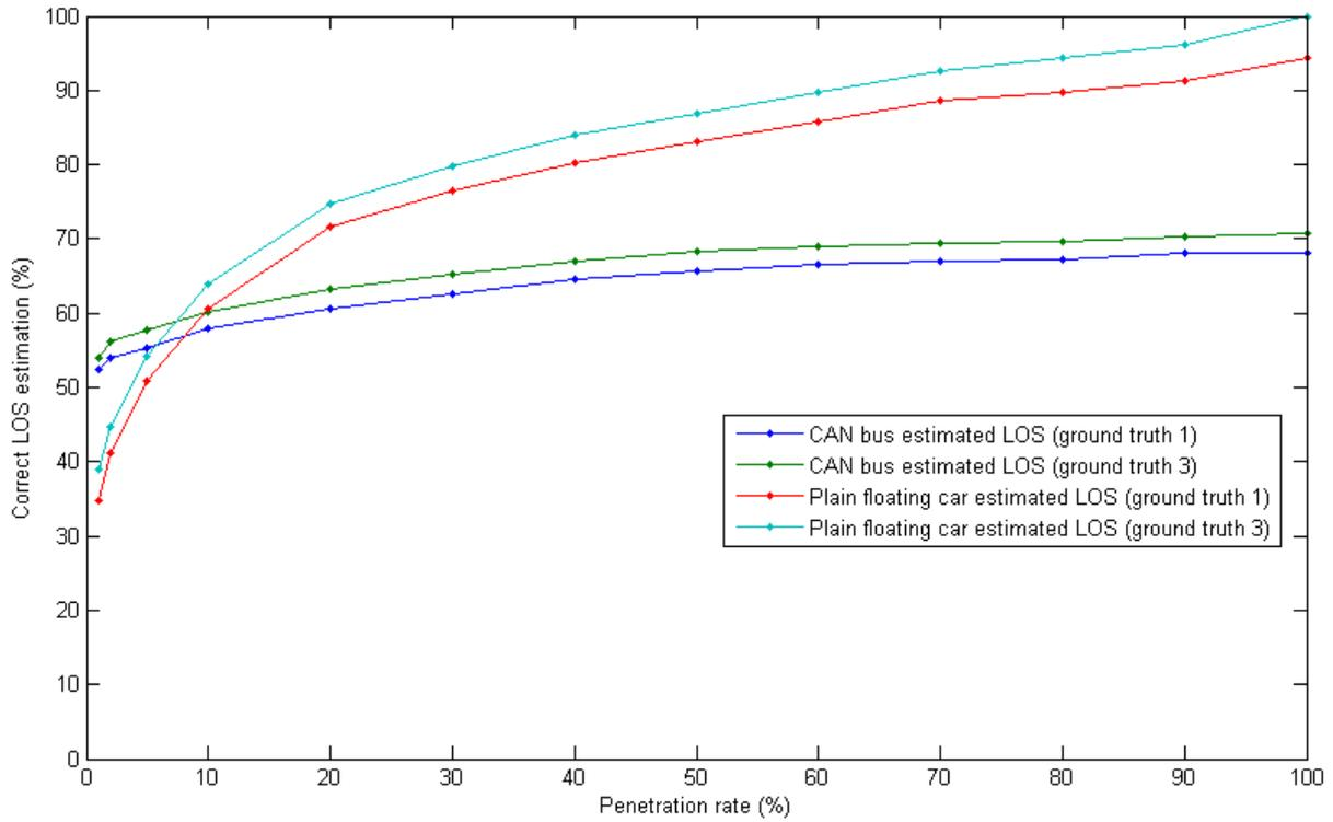
Figure 31: Penetration rate versus correct LOS estimation with simulated plain floating car data (containing only positional data) and average simulated CAN bus speed, for ground truth 1, determined with simulation loop detector data, and ground truth 3, determined with the vehicle presence, for minutes with available data.
