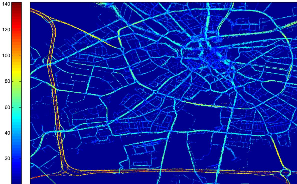
Figure 56: Average speed (km/h) in Eindhoven. The color scale represents the average speed of the uCAN equipped vehicles at a specific location. Dark blue (the background color) indicates that no vehicles in the data set have been at that location. Blue indicates that the average speed of the vehicles at the location is low. Red indicates that the average speed of the vehicles at the location is high.
