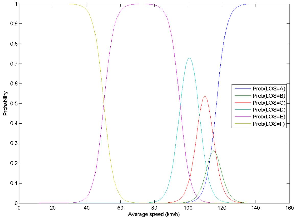
Figure 86: LOS probability functions for 100% penetration
