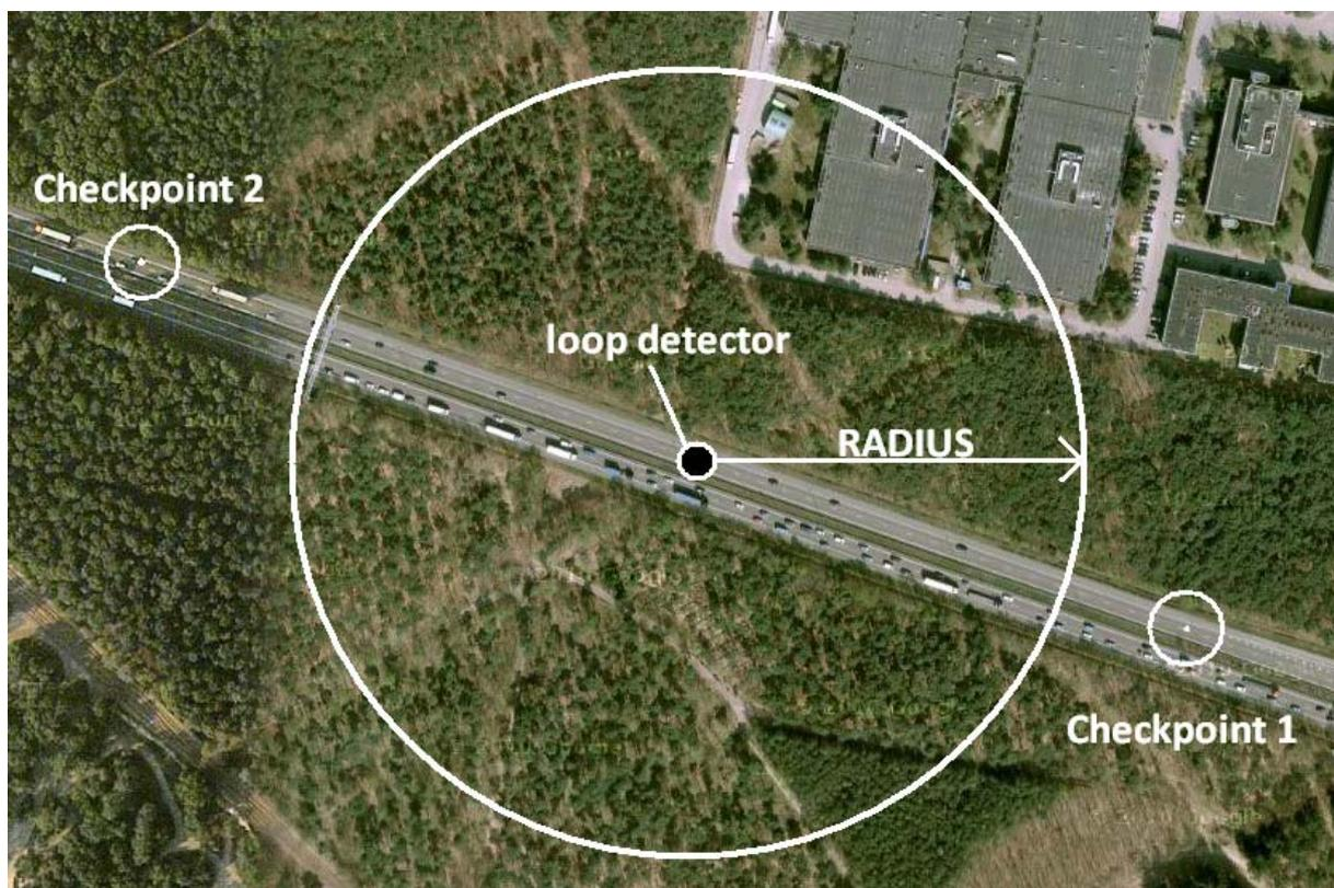
Figure 6: CAN bus data filtering. uCAN equipped vehicles are checked for subsequently passing checkpoint 1 and checkpoint 2 with their GPS data. When they do, it is certain they are driving on the motorway and in the correct direction. From the CAN bus data points between both checkpoints, the ones which are within the radius of one of the loop detectors (just one in the figure) are stored and can be used to combine with the loop detector data.
