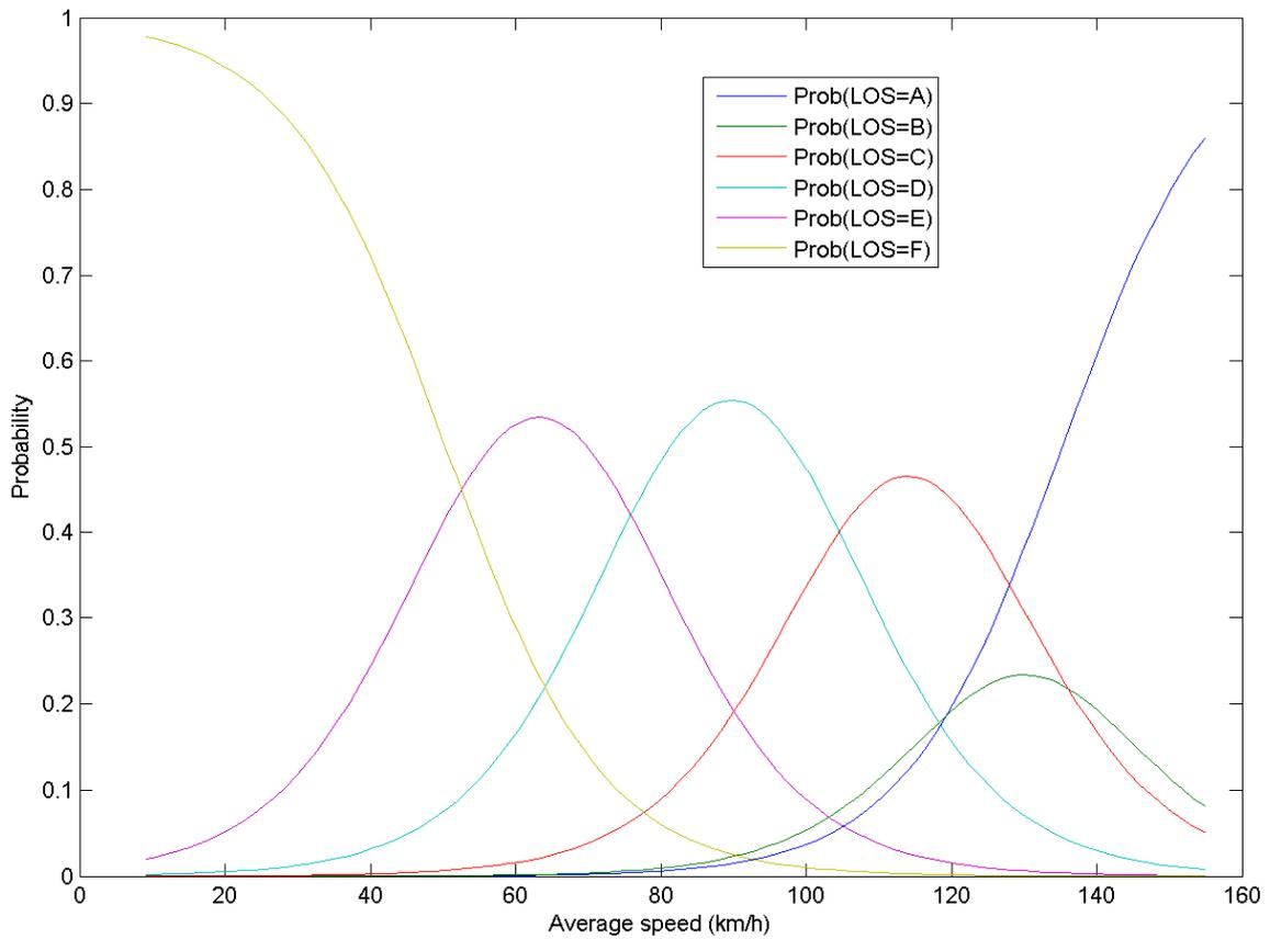
Figure 73: LOS probability functions (LOS ground truth 4)
