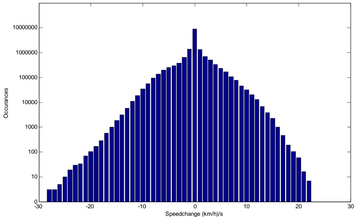
Figure 62: Occurrences of the change in CAN bus speed in subsequent seconds, without outliers
