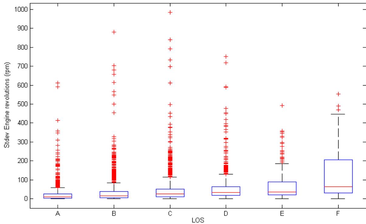
Figure 20: LOS versus st.dev of the engine rotational speed. The standard deviation of the engine rotational speed of the uCAN equipped vehicles passing a loop detector is plotted against the Level of Service ground truth in the corresponding minute.
