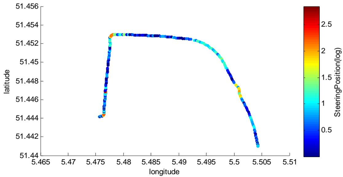
Figure 47: Position and log adjusted steering position during the trip. The (logarithmic) color scale indicates the difference between the steering position and the neutral steering position.
