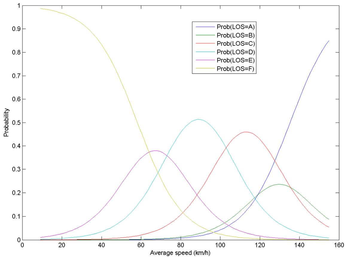
Figure 71: LOS probability functions (LOS ground truth 2)
