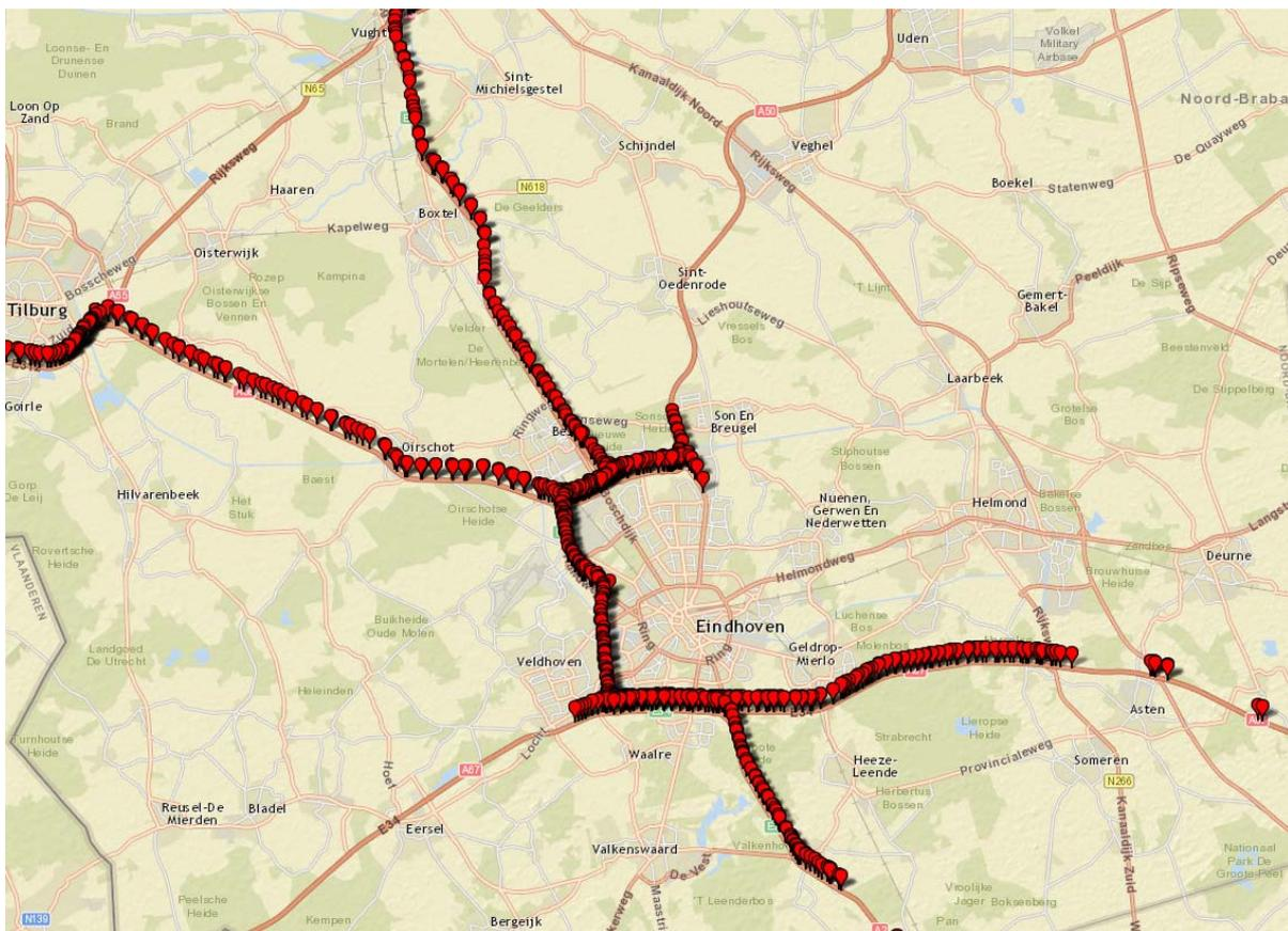
Figure 4: Detection loops in the Eindhoven area. The red icons indicate the locations of the loop detectors.
