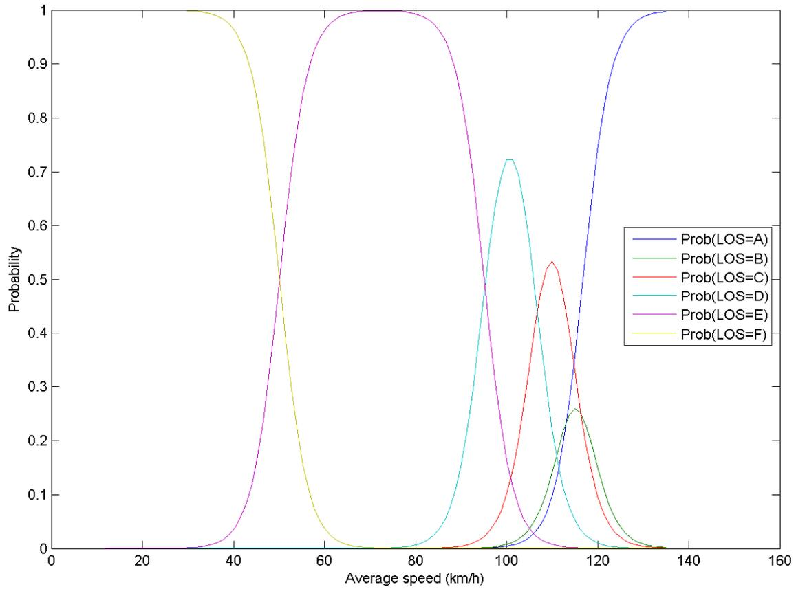
Figure 84: LOS probability functions for 80% penetration
