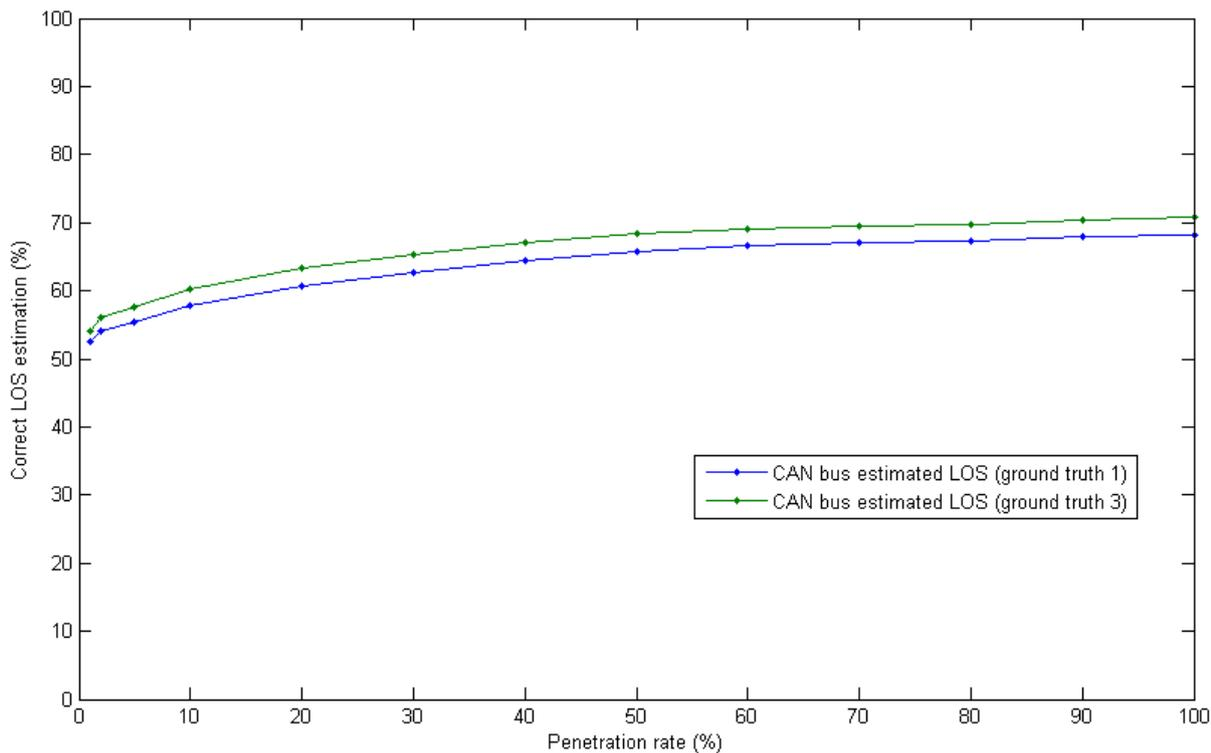
Figure 26: Penetration rate versus correct LOS estimation with simulated average CAN bus speed, for ground truth 1, determined with simulation loop detector data, and ground truth 3, determined with the vehicle presence, for minutes with available data.
