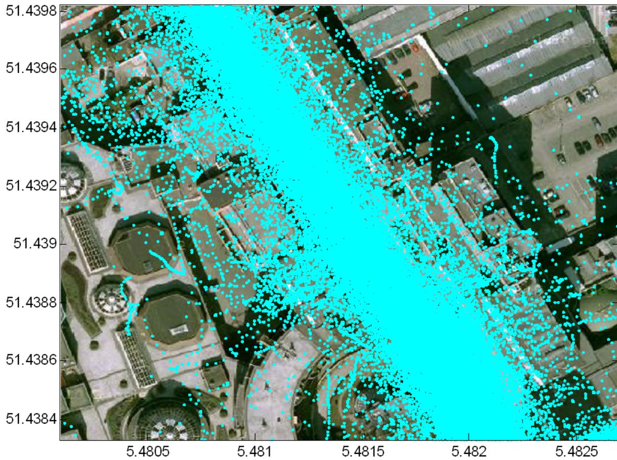
Figure 64: GPS positions at the Vestdijk, Eindhoven. The blue dots represent the recorded positions of the uCAN equipped vehicles in the data set.
