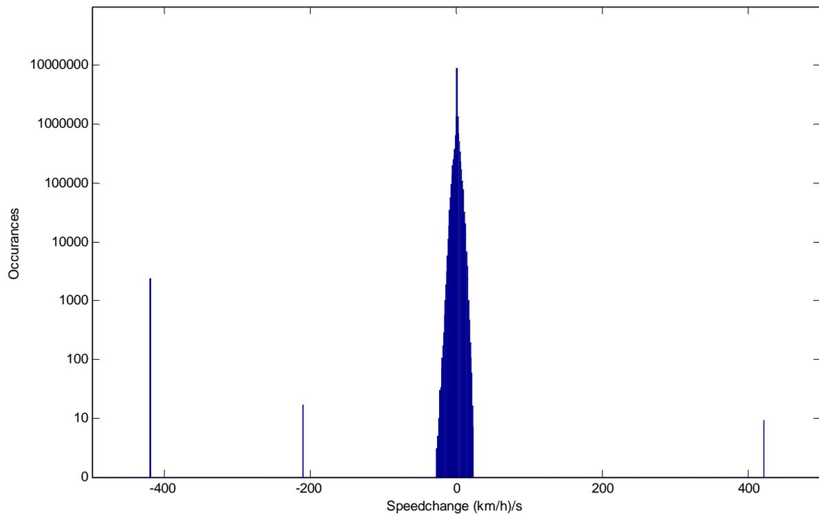
Figure 61: Occurrences of the change in CAN bus speed in subsequent seconds
