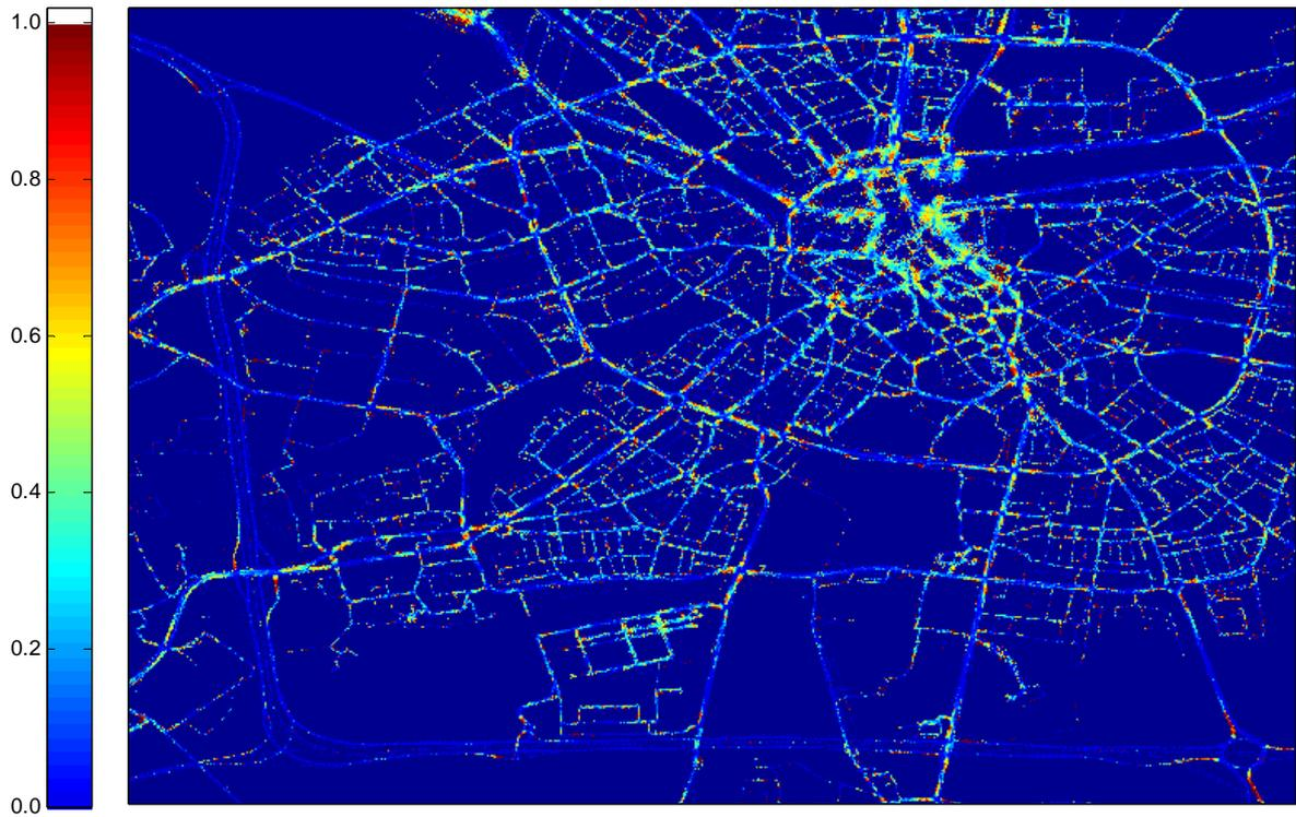
Figure 57: Brake usage in Eindhoven. The color scale represents which part of the uCAN equipped vehicles uses its brakes while being at a specific location. Dark blue (the background color) indicates that no vehicles in the data set have been at that location. Blue indicates that no vehicles use their brakes at the location. Red indicates that all vehicles use their brakes at the location.
