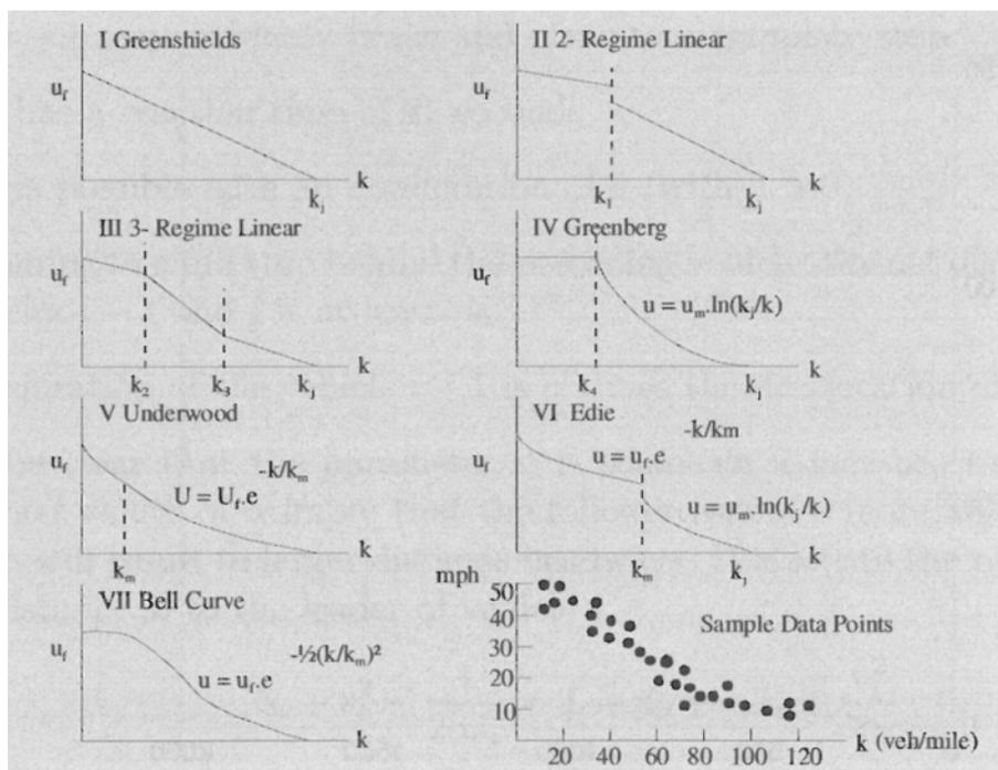
Figure 8: Fundamental diagram models [20]
