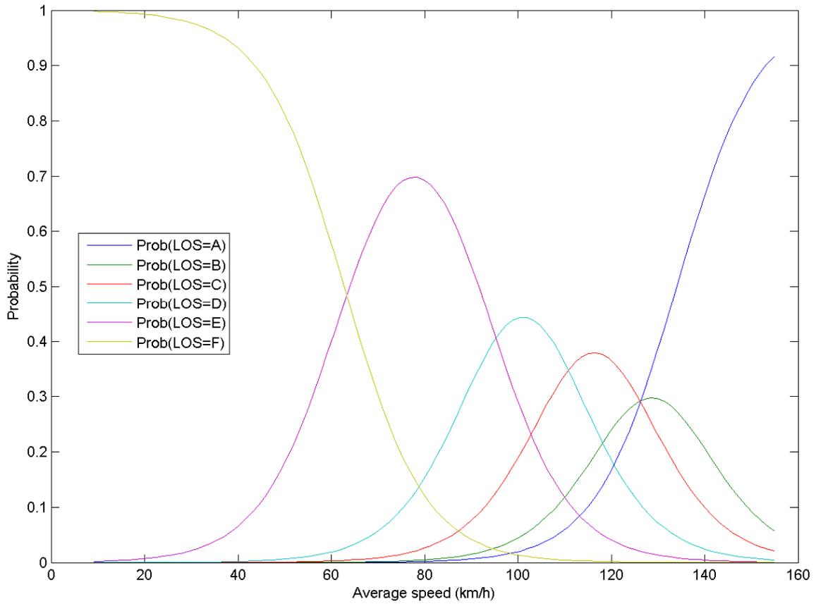
Figure 72: LOS probability functions (LOS ground truth 3)
