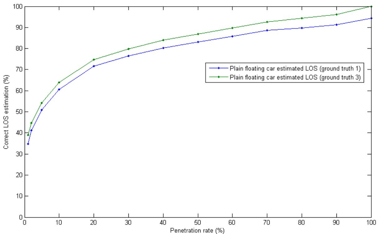
Figure 29: Penetration rate versus correct LOS estimation with simulated plain floating car data (containing only positional data), for ground truth 1, determined with simulation loop detector data, and ground truth 3, determined with the vehicle presence, for minutes with available data.
