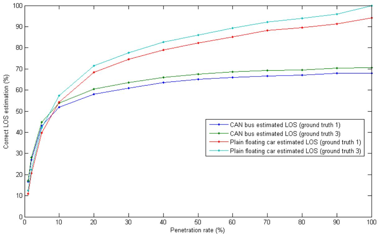
Figure 32: Penetration rate versus correct LOS estimation with simulated plain floating car data (containing only positional data) and average simulated CAN bus speed, for ground truth 1, determined with simulation loop detector data, and ground truth 3, determined with the vehicle presence, for all minutes.
