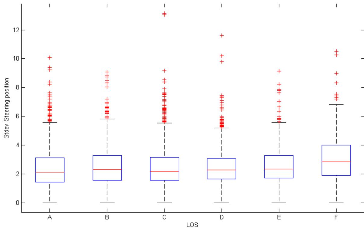
Figure 17: LOS versus st.dev of steering position. The standard deviation of the steering position of the uCAN equipped vehicles passing a loop detector is plotted against the Level of Service ground truth in the corresponding minute. The unit of steering position is unknown.
