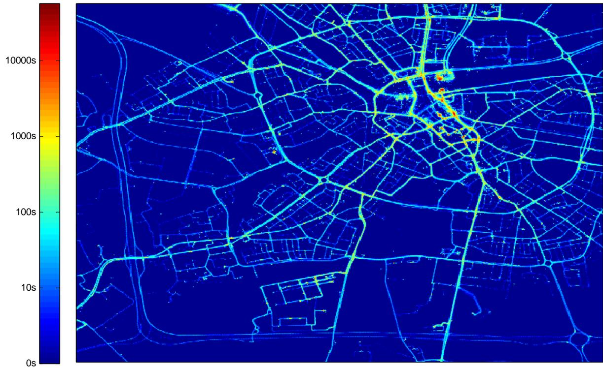
Figure 55: Presence of the uCAN equipped taxis in Eindhoven. The color scale represents how often a uCAN equipped vehicle was present at a specific location. Dark blue (the background color) indicates that no vehicles in the data set have been at that location. Blue indicates that vehicles were rarely present at the location. Red indicates that vehicles were often present at the location.
