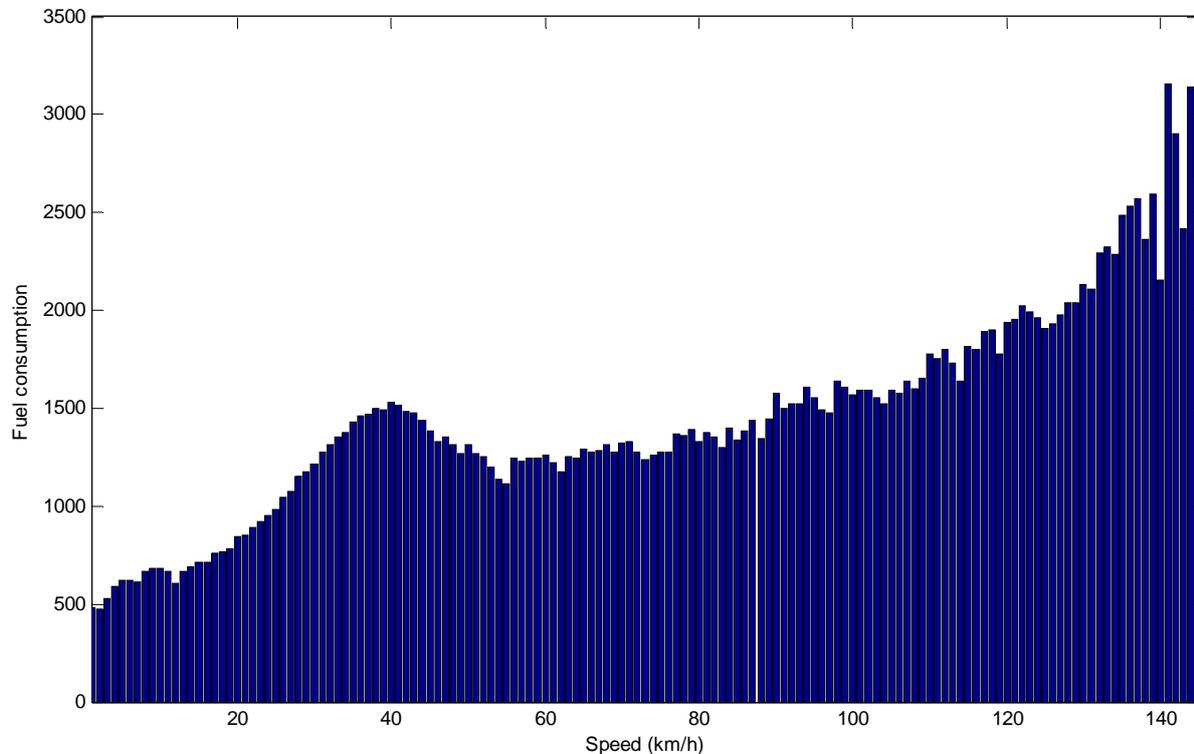
Figure 54: Speed versus average fuel consumption. The unit of the fuel consumption is unknown.
