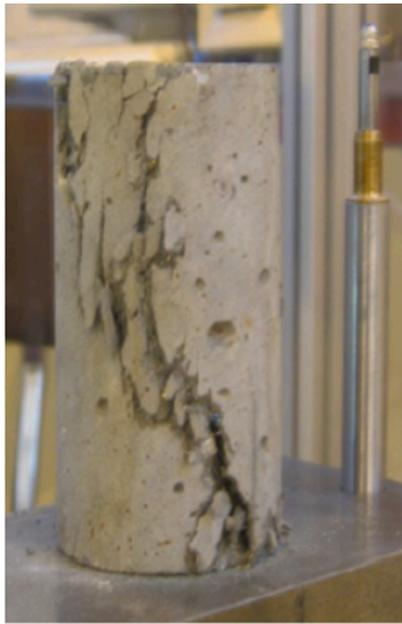
(a) Failure mode of UHPCFRC
