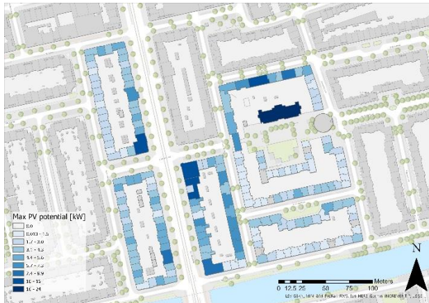
Figure 18: Maximum PV capacity case study area Diamantbuurt [kW].
