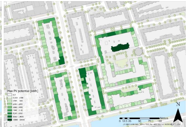
Figure 19: Maximum yearly PV energy yield case study area Diamantbuurt [kWh].
