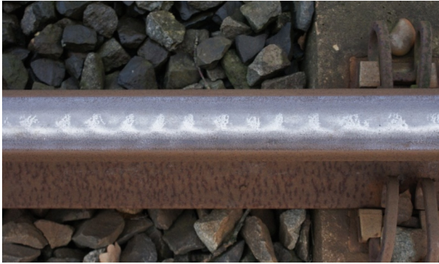
Fig. 1. Short pitch Corrugation observed in the Dutch railway with a wavelength of approximately 30 mm.
