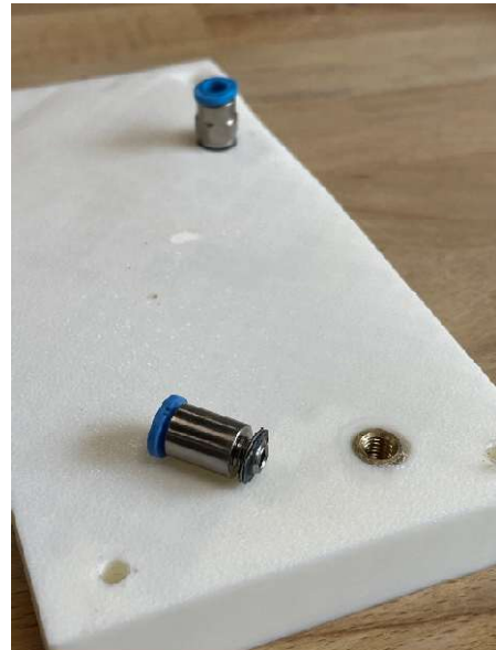
Figure 79: Festo air connector and insert in top plate
