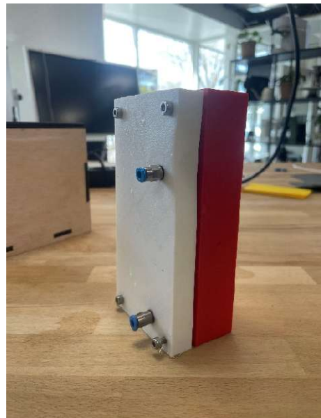
Figure 80: Lab Setup of Venturi V1, see the warping of PLA
