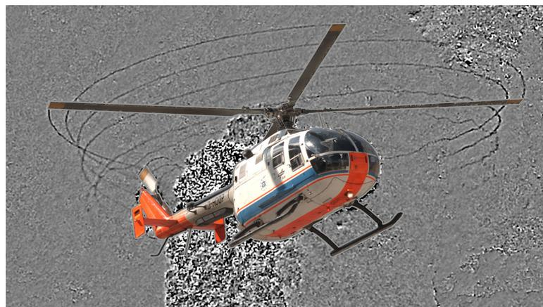
Figure 6.14: Vorticity pattern about a Bo 105 during a swinging maneuver [83]
