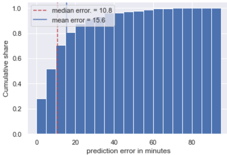
Figure 8.7: Absolute error distribution after applying a MLP Regression to fit M1's expected number of presences of the several access types to the DHS cluster average travel time
