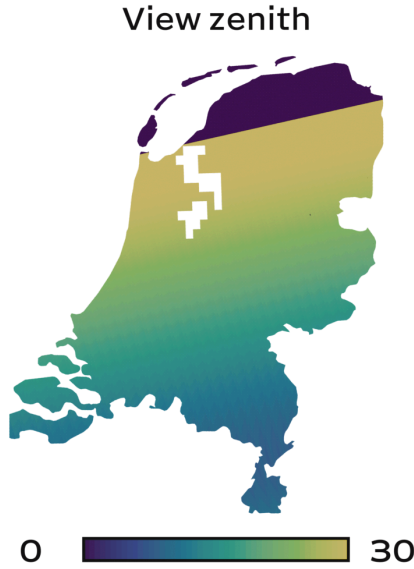
Figure 1: An example of the view zenith data for an LST image. The shifting colors indicate what the angle of that position was relative to the ISS. The values are in degrees.
