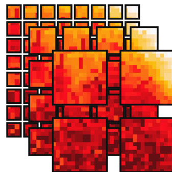
Figure 7: A simplified representation of how a SWIN transformer processes images at changing patch density.
