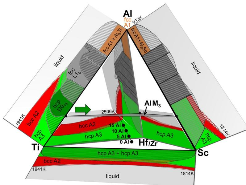
**Figure 2.** 3D representation of the multi-component phase diagram constructed from the binary diagrams (Fig. 1). For visualization purposes, the Zr-binary phase diagrams (similar to the ones of Hf, see Fig. 1) are not shown. Black filled circles indicate the phase diagram trajectory for varying Al-concentration including the main alloy for the ab initio and experimental investigations with 15 at.% Al.
