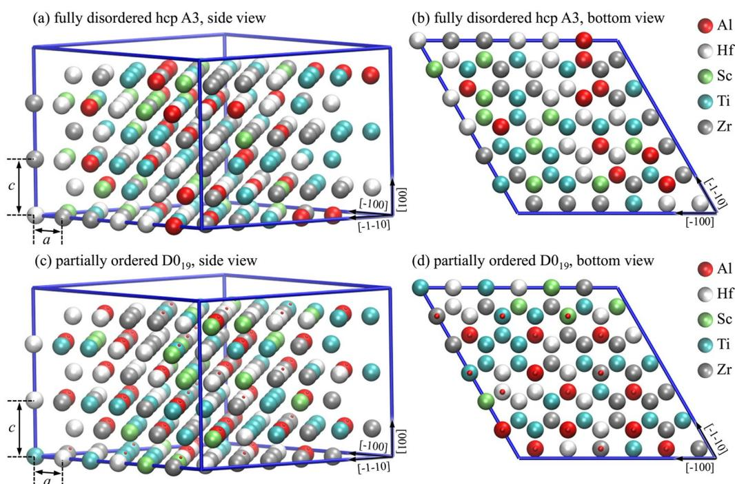
**Figure 3.** Side and bottom view of the 216-atom super cells of the disordered hcp A3 structure [(a) and (b)] as well as for the partially ordered D0<sub>19</sub> structure [(c) and (d)] employed in the first-principles calculations for Al<sub>15</sub>Hf<sub>25</sub>Sc<sub>10</sub>Ti<sub>25</sub>Zr<sub>25</sub> at.%. The small red dots in (c) and (d) indicate the sublattice positions for the ordered Al atoms in the D0<sub>19</sub> superstructure.
