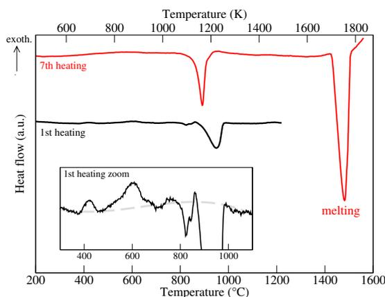
**Figure 7.** DTA heat flow curves of the  $\text{Al}_{15}\text{Hf}_{25}\text{Sc}_{10}\text{Ti}_{25}\text{Zr}_{25}$  at.% HEA. The black curve corresponds to the 1<sup>st</sup> heating cycle directly after casting. The red curve shows the 7<sup>th</sup> heating cycle which corresponds to the equilibrated situation, i.e., further heating cycles show the same dependence. The inset enlarges the 1<sup>st</sup> heating curve and the gray dashed line is a guide to the eye indicating the baseline.
