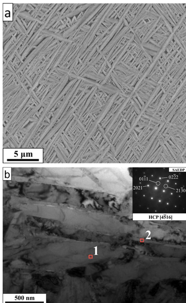
**Figure 5.** Microstructure of the  $\text{Al}_{15}\text{Hf}_{25}\text{Sc}_{10}\text{Ti}_{25}\text{Zr}_{25}$  at.% HEA in the as-cast state; (a) SEM image, (b) TEM-BF with SAED patterns and EDS point analysis taken at the red squares, with the results given in Table 3.
