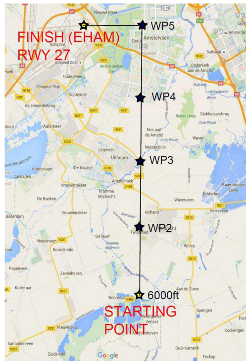
Figure 17. Flight track with waypoints towards runway 27 at Schiphol airport, source: Google Maps
