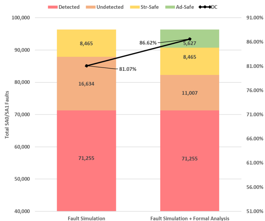
Figure 10. Combined results in CPU: uptrend in DC when fault simulation and formal analysis combined.
