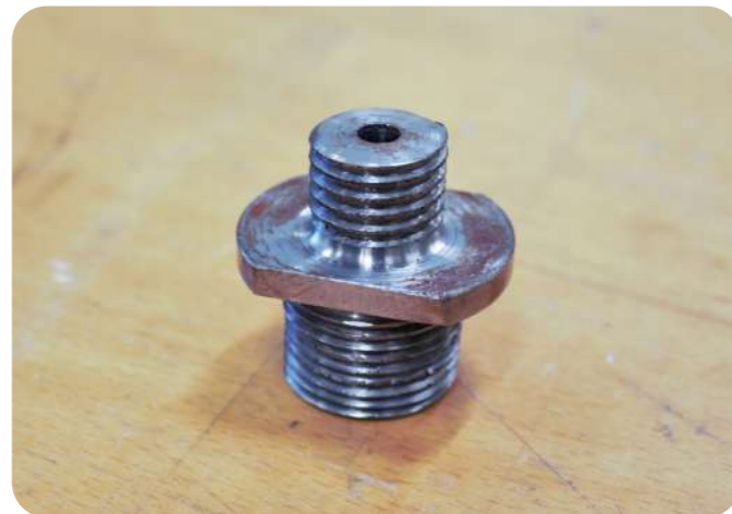
Figure 87: Lathed nozzle connector
