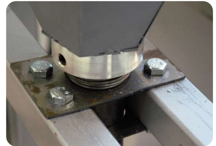
Figure 104: Bent support plate
