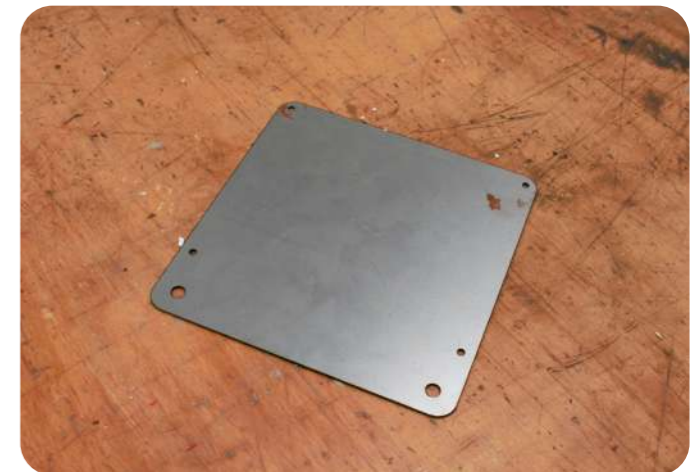
Figure 97: A piece of lasercut sheetmetal
