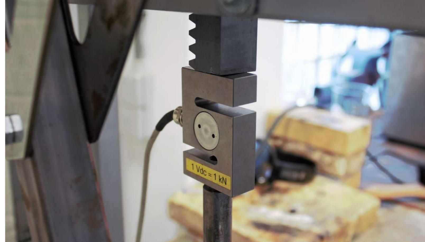
Figure 91: Force sensor between rack and plunger
