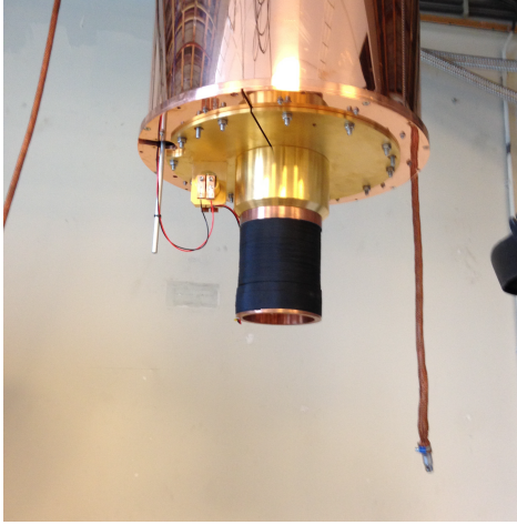
Figure 3.13: Magnet is thermalized to the 3 K stage. As a puck is inserted, the puck is located slightly above inside the solenoid.
