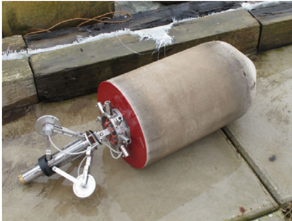
Figure 3.8: Photograph of the ultrasound tool used in the tests attached to a foam pig. Courtesy of Applus RTD.
