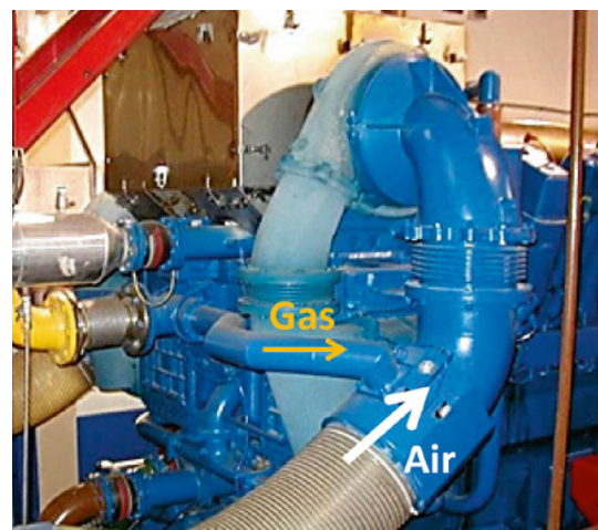
Figure 2.12: Homogeneous charged gas engine; gaseous fuel injection before turbocharger [39].
