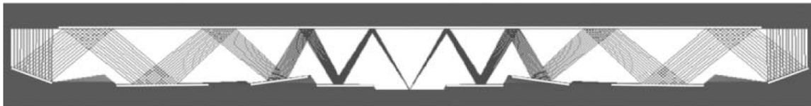
Figure 9.2: Example of an 8-times folded annular optic [2]
