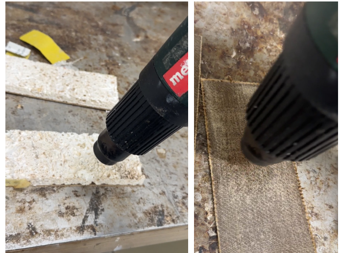
Figure 77: left, heating the surface of the core; right, heating the surface of the flax fibers
