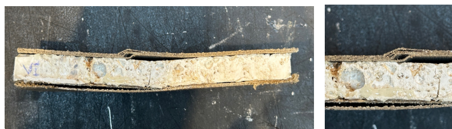
Figure 110: Images of PLAX B5. Left; Image after the testing testing; Right, close up where the material has failed.
