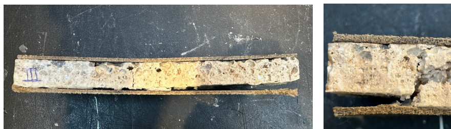
Figure 108: Images of PLAX B3. Left; Image after the testing testing; Right, close up where the material has failed.
