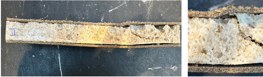
Figure 106: Images of PLAX B1. Left; Image after the testing testing; Right, close up where the material has failed.
