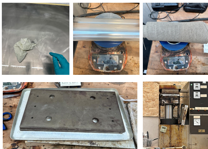
Figure 73: Process images of the film stacking method II B
