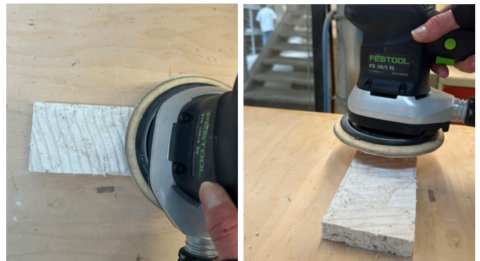
Figure 75: electrical sandpaper machine and the texture of the core
