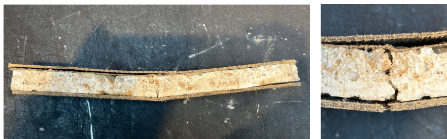
Figure 109: Images of PLAX B4. Left; Image after the testing testing; Right, close up where the material has failed.
