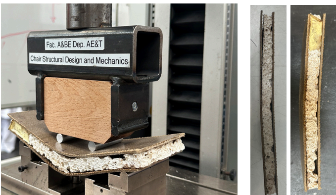
Figure 104: PLAX A4. Left, during testing. Right, after testing images
