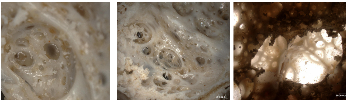
Figure 115: Microscope images showing the cellular structure of the foam material
