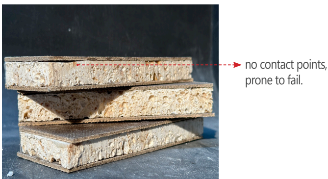
Figure 99: PLAX B samples bonded with two component binder.
