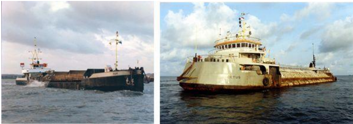
Figure 2-16 Side dumping vessels; Photograph Royal Boskalis Westminster
