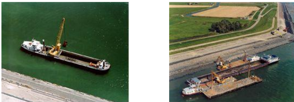
Figure 2-17 Left: Crawler crane on rails. Right: Back hoe on ship; Photograph L. Paans &amp; Zonen
