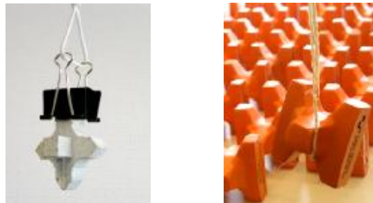
Figure 4-11 Left; Xbloc placed by hydraulic clamp Right; Accropode placed by sling
