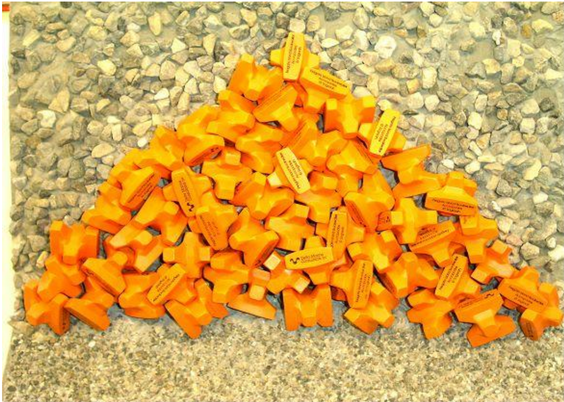
Figure 8-10 Placement of Accropode for experiment DMC March 2004
