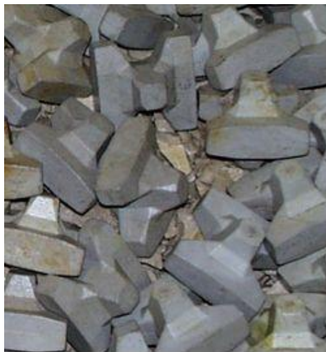
Figure 8-11 Incorrect density and loose units
