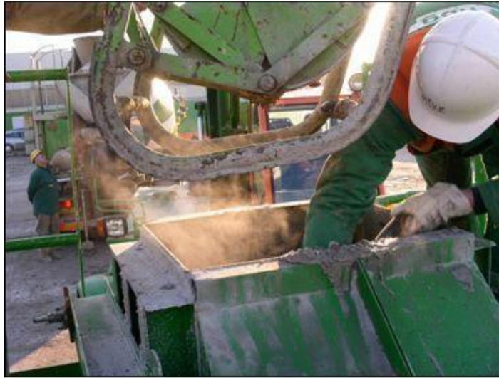
Figure 2-9 Pouring of concrete in mould.
