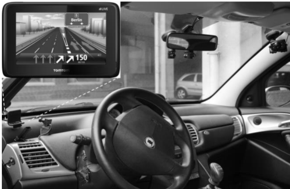
Figure 7.A1: Vehicle cabin layout (Lancia Ypsilon), including a navigation system photo. The navigation system mount is installed to the left of the steering wheel, with a camera facing it. In the Peugeot 207 the system was mounted to the right of the steering wheel.
