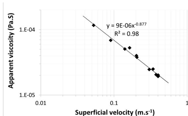
**Figure 7a** Measured apparent viscosity of the foam as a function of the total superficial velocity
