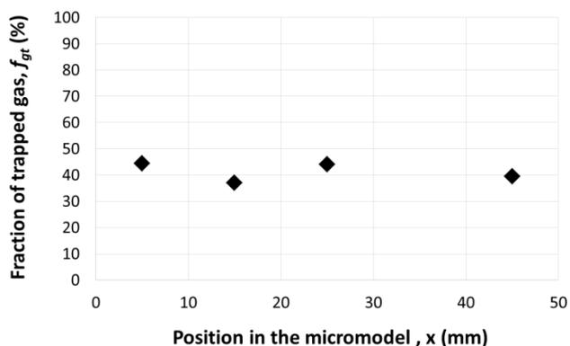
**Figure 4** Trapped gas fraction as a function of position in the micromodel. Positions are defined with respect to the inlet of the micromodel. The measurements were carried out with a foam quality of 0.3 and a superficial velocity of  $0.14 \text{ m.s}^{-1}$ .
