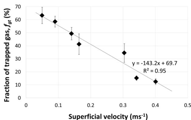
**Figure 5** Trapped gas fraction as a function of the flow rate in the micromodel. Foam quality varies from 0.94 for the lowest flow rate to 0.98 for the highest flowrate. The error bars indicate the range of values obtained with small variations in the velocity thresholding.
