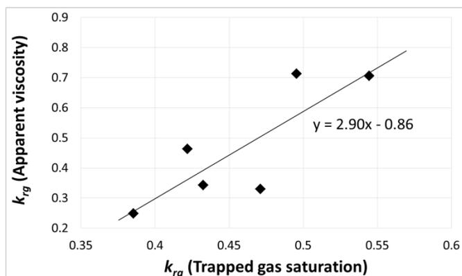
**Figure 10** Gas relative permeability  $k_{rg}$  calculated from the foam apparent viscosity  $\mu_{foam}$  (equation 5) plotted as function of  $k_{rg}$  calculated from the trapped gas  $S_{gt}$  (equation 3).
