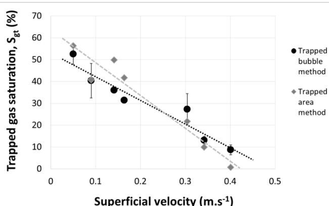
**Figure 9** Trapped gas saturation, measured using the trapped area and the trapped bubble techniques, plotted as a function of the superficial velocity. The error bars in the trapped bubble fraction measurements indicate the range of values obtained with small variations in the velocity thresholding.
