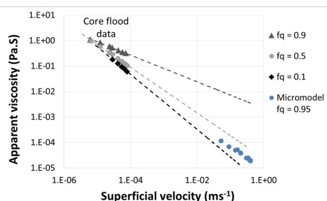
**Figure 7b** Extended version of the shear thinning curve, including data from shear thinning tests carried out locally in Bentheimer sandstone cores<sup>15</sup>.
