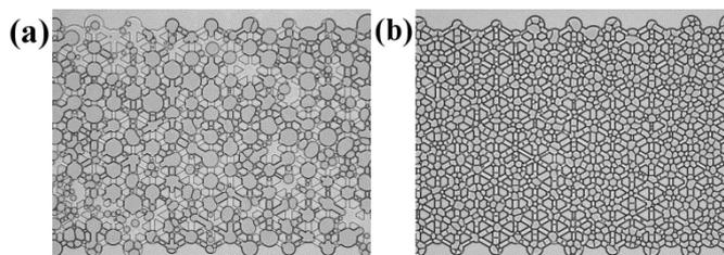
**Figure 6** Images of the bubbles in the porous media for a) linear velocity of  $0.09 \text{ m.s}^{-1}$  and b)  $0.4 \text{ m.s}^{-1}$ . There is a strong dependence of foam structure on the flow velocity. Average bubble size decreases with increasing velocity.
