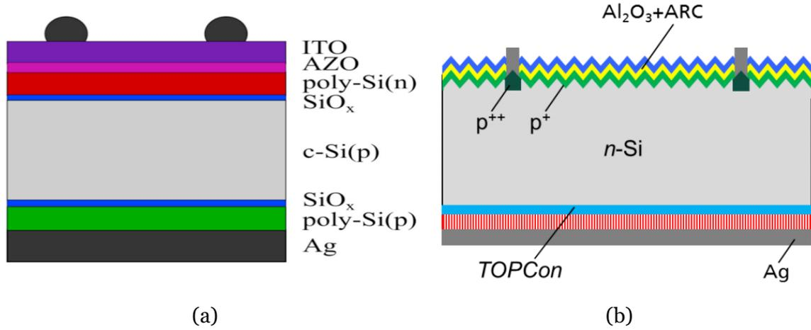
Figure 1.8: Schematic sketches of (a) top/rear poly-Si/SiO<sub>x</sub> contacts solar cell; (b) TOPCon solar cell.
