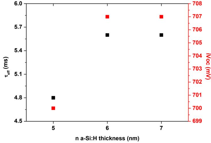
Figure 3.6: Effect of n-type a-Si:H thickness on lifetime ( $\Delta=10^{15} \text{ cm}^{-3}$ ) and  $iV_{OC}$ . Measured on symmetric structures with fixed 4.5 nm i a-Si:H and different n a-Si:H thickness after 190 °C 30 min annealing on oven.
