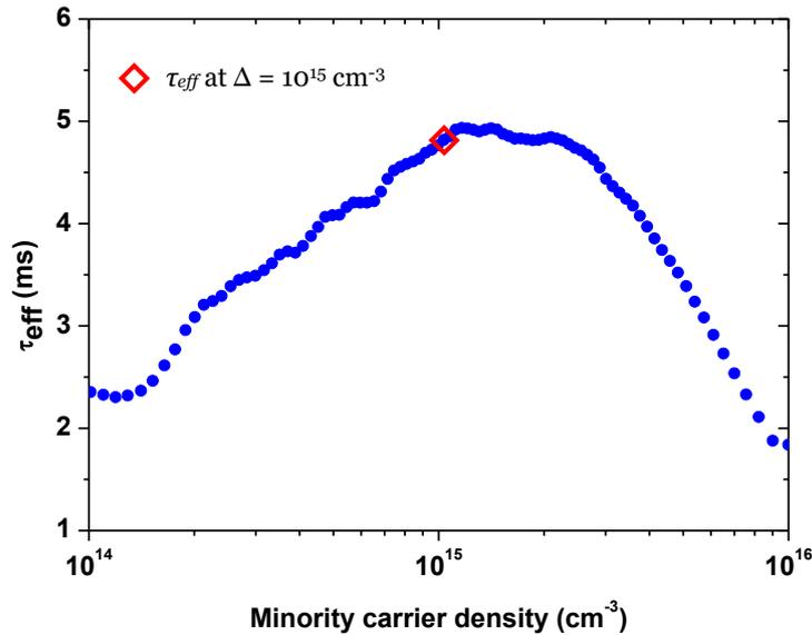
Figure 2.5: Effective minority carrier lifetime of FZ n-type c-Si wafer passivated by 20 nm i a-Si:H on both sides after 190 °C annealing in air for 30 min as a function of excess carrier density.
