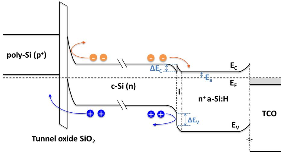
Figure 1.11: Schematic band diagram of poly-Si ( $p$ )/ $\text{SiO}_2$ /c-Si ( $n$ )/a-Si:H ( $i$ )/a-Si:H ( $n^+$ )/TCO structure of hybrid solar cells
