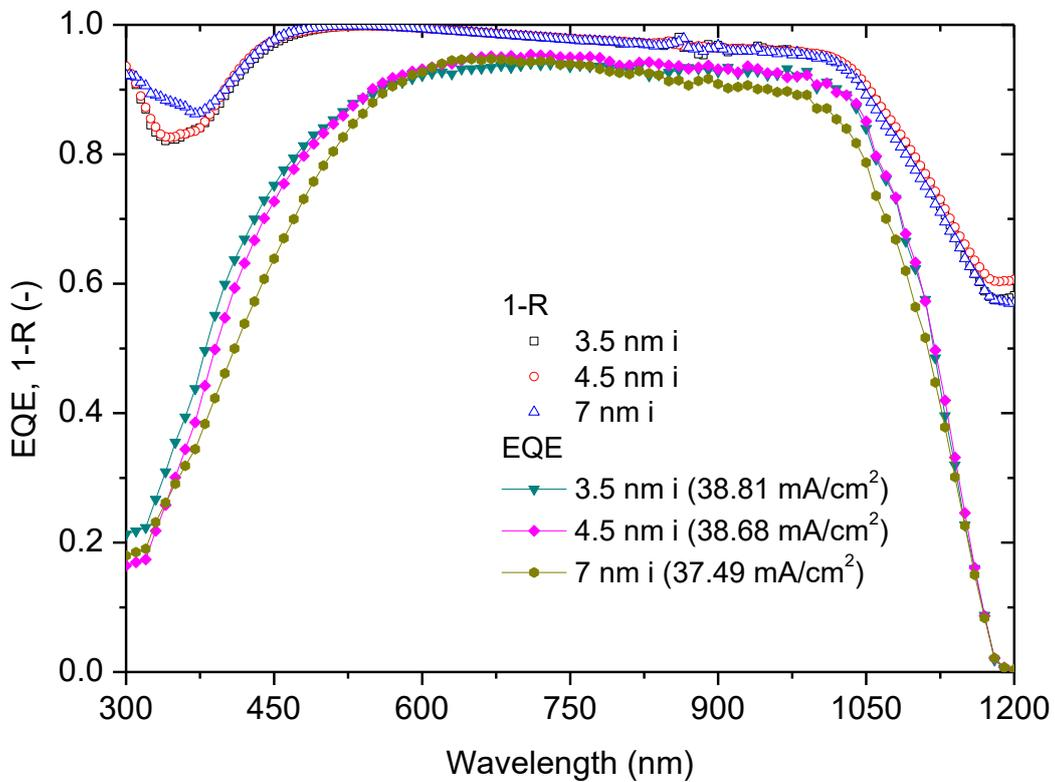
Figure 3.8: 1-R and EQE spectra of hybrid solar cells with different intrinsic a-Si:H thickness.
