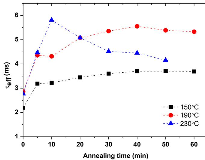
Figure 3.6: Lifetime at  $\Delta=10^{15} \text{ cm}^{-3}$  and implied- $V_{oc}$  as the functions of post-deposition annealing time and temperature on symmetric structures with fixed 4.5/6 nm i/n layers. The annealing was carried out in air environment on oven.
