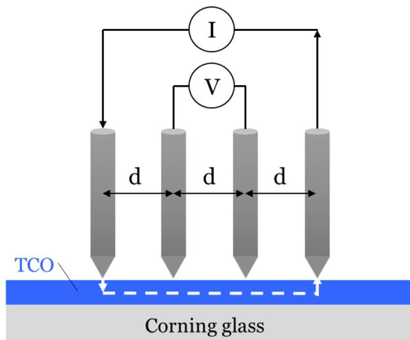
Figure 2.7: Schematic sketch of four-point probe measurement.
