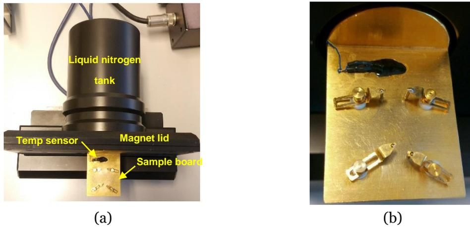
Figure 2.6: Sample mounting fixture: (a) with upper cooling reservoir; (b) zoom-in of sample stage.
