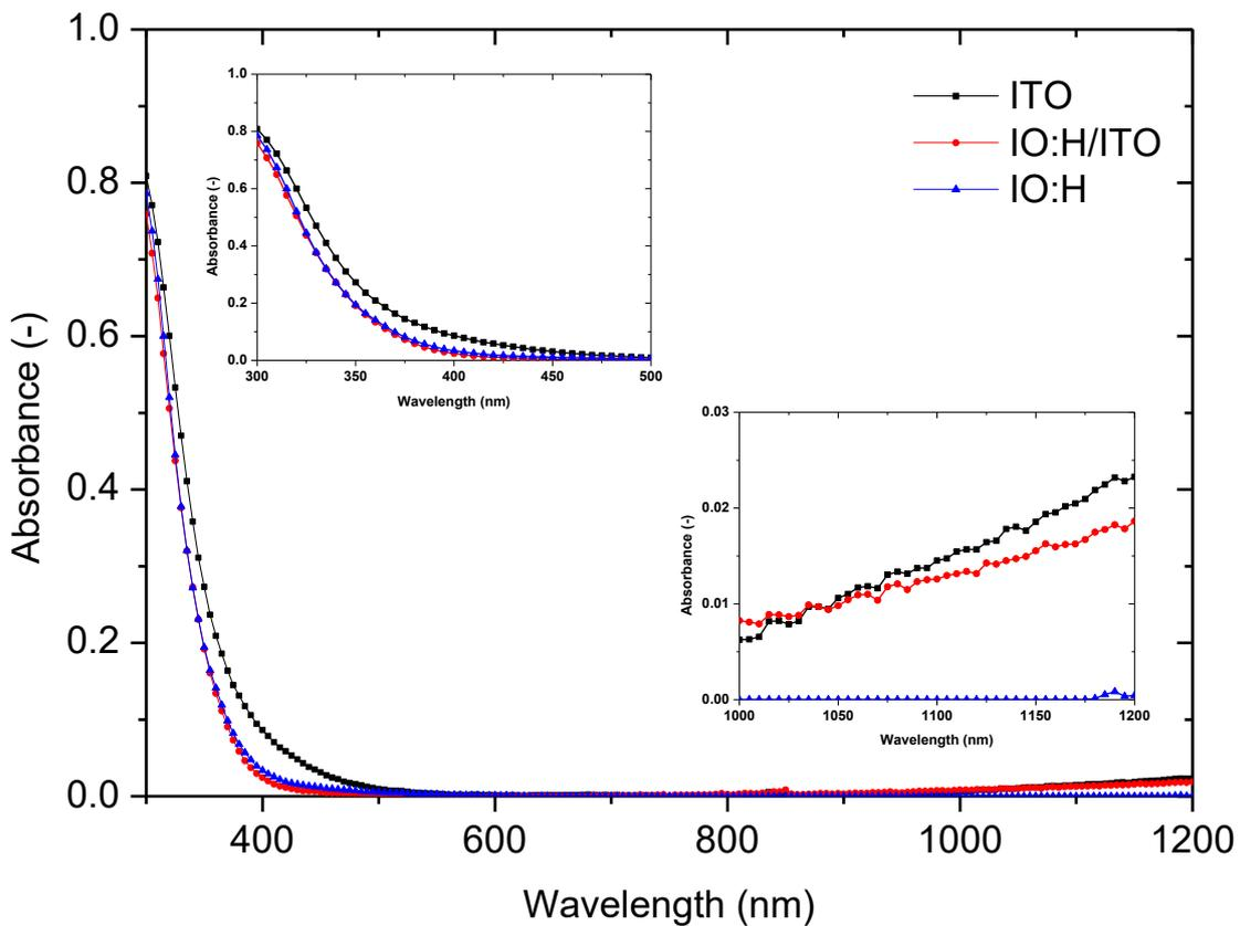
Figure 4.5: Absorption spectra for ITO (annealed 30 min @ 190 °C in air), IO:H/ITO stacks (IO:H film annealed 30 min @ 180 °C in vacuum) and IO:H (annealed 30 min @ 180 °C in vacuum), calculated by  $1-R-T$ . Insets are presented in the plot to highlight the short-wavelength and NIR part of the spectrum. IO:H was used as a reference.
