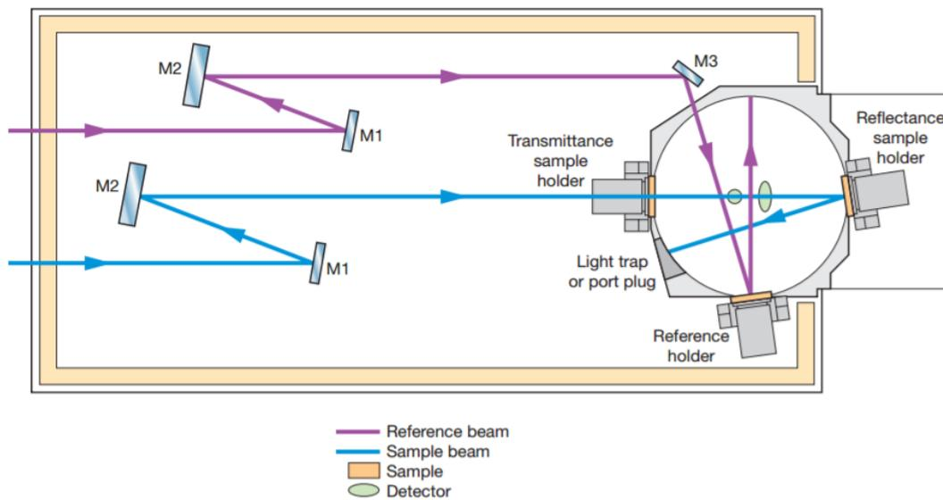
Figure 2.9: Top view of 150 mm integrating sphere (IS) and its optical design [55].
