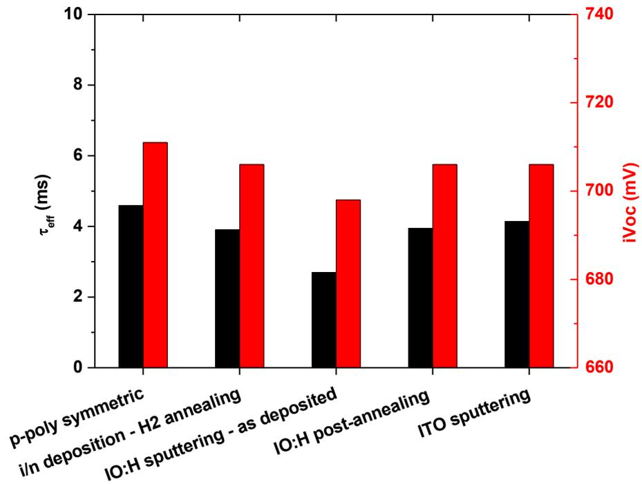
Figure 4.6: Lifetime at  $\Delta=10^{15} \text{ cm}^{-3}$  and  $iV_{\text{oc}}$  for different process steps during precursor cells fabrication: (a) cell #1 with ITO; (b) cell #2 with IO:H/ITO stacks. Measured in Sinton lifetime tester. Optical constant values were set as 0.7/0.8 for the structures without/with TCO respectively.
