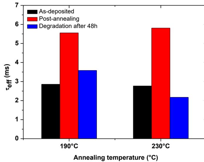
Figure 3.7: Lifetime at an injection level of  $\Delta=10^{15} \text{ cm}^{-3}$  on symmetric structures with 190 °C and 230 °C annealing temperatures at three different stages: as-deposited, post-deposition annealing and degradation after 48h.
