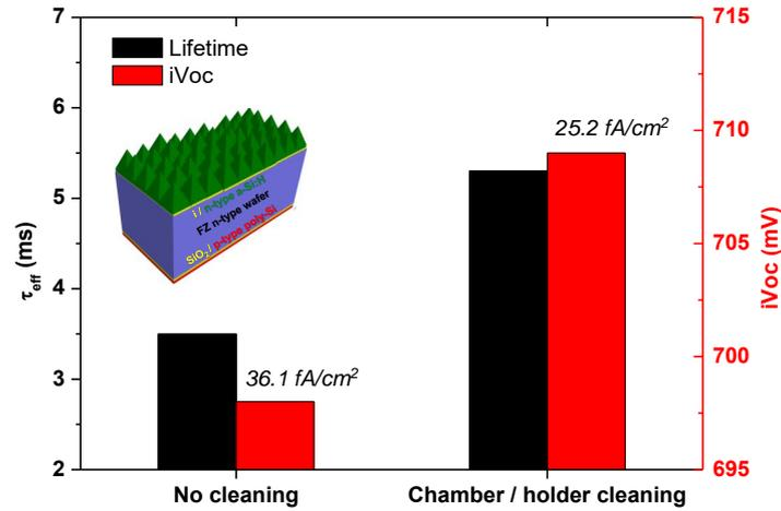
Figure 3.5: Lifetime ( $\Delta=10^{15} \text{ cm}^{-3}$ ),  $iV_{oc}$  and  $J_0$  measurements on precursor cells (7/6 nm i/n a-Si:H stacks as FSF) without/with chamber cleaning and holder deposition. Measured after 190 °C 30 min annealing on oven.
