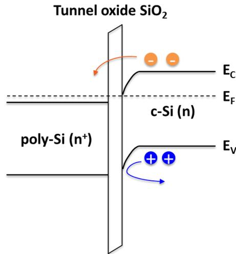
Figure 1.9: Schematic band diagram of  $n^+$  poly-Si/SiO<sub>x</sub> passivating contact.
