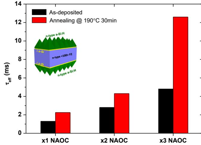
Figure 3.4: Effective minority carrier lifetime ( $\Delta=10^{15} \text{ cm}^{-3}$ ) on symmetric structures with different NAOC cleaning times.
