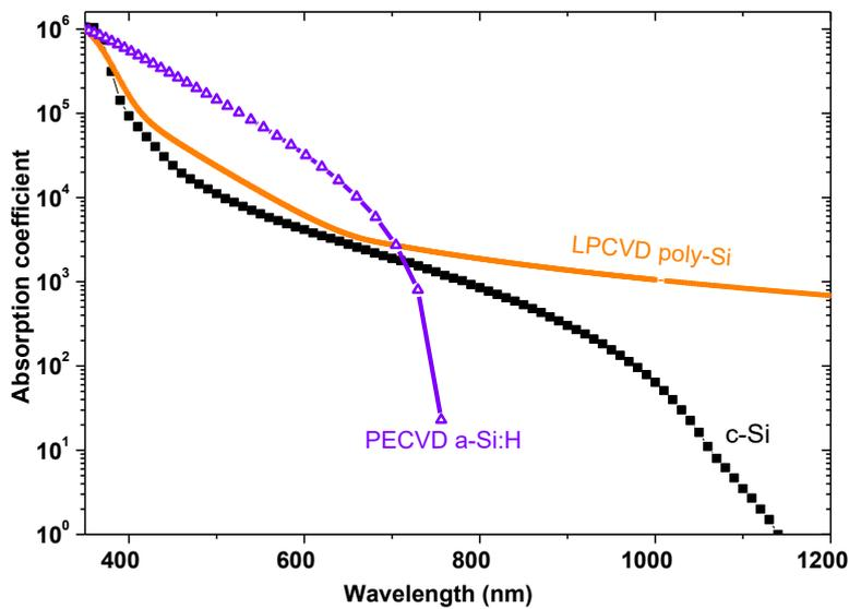
Figure 3.2: Absorption coefficient of PECVD a-Si:H, LPCVD poly-Si and c-Si.
