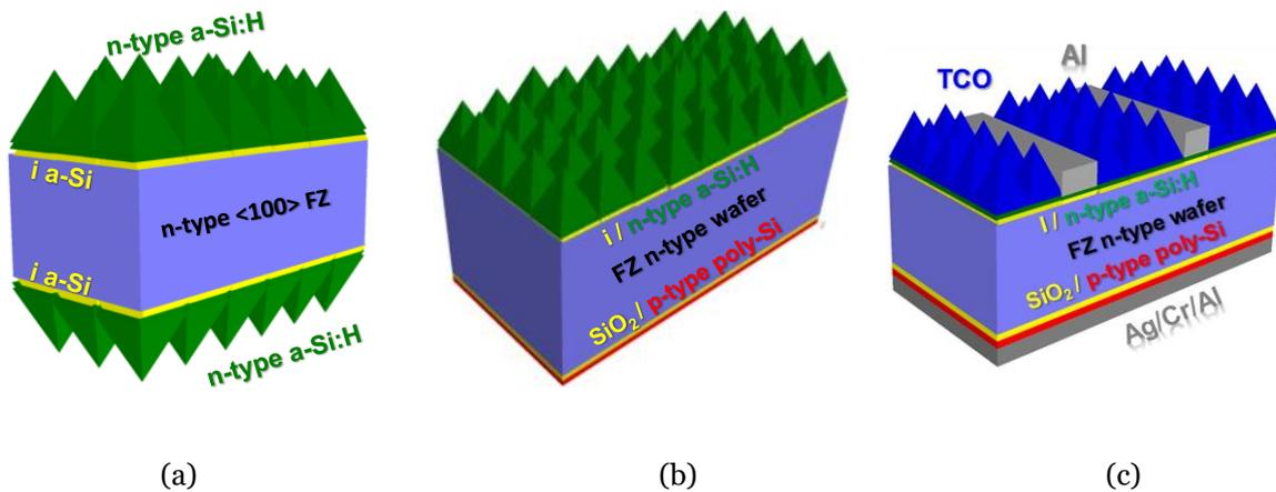
Figure 3.3: Schematic sample structures on n-type c-Si FZ wafer: (a) symmetric structure with i/n a-Si:H layers on both-side textured surfaces; (b) a precursor cell with i/n a-Si:H layers on front textured surface and SiO<sub>x</sub>/poly-Si films on rear flat surface; (c) a complete hybrid solar cell.
