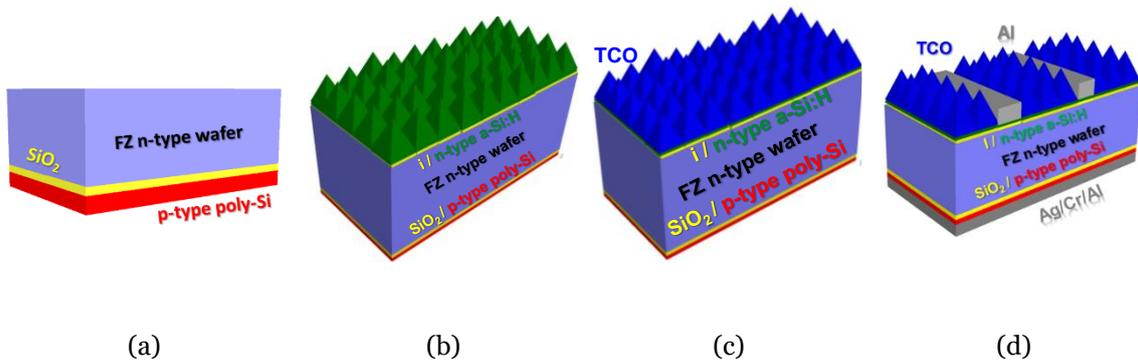
Figure 2.3: Process flowchart of hybrid solar cells: (a) carrier-selective passivating rear emitter (SiO<sub>2</sub>/p poly-Si); (b) heterojunction front surface field (i/n a-Si:H); (c) front transparent conductive oxide (TCO); (d) front and rear metal contacts.
