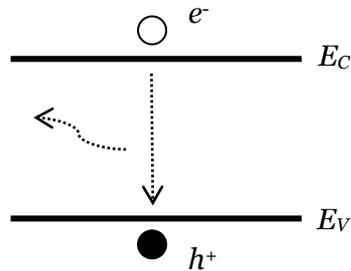
Figure 1.2: Radiative recombination in bulk semiconductors.
