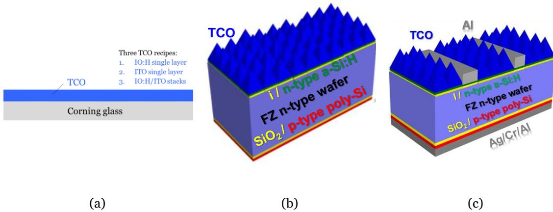
Figure 4.2: Schematic sample structures: (a) glass sample with TCO layers; (b) a precursor cell with TCO/a-Si:H (n/i) layers on front textured surface and SiO<sub>x</sub>/poly-Si (p) films on rear flat surface; (c) a complete hybrid solar cell.
