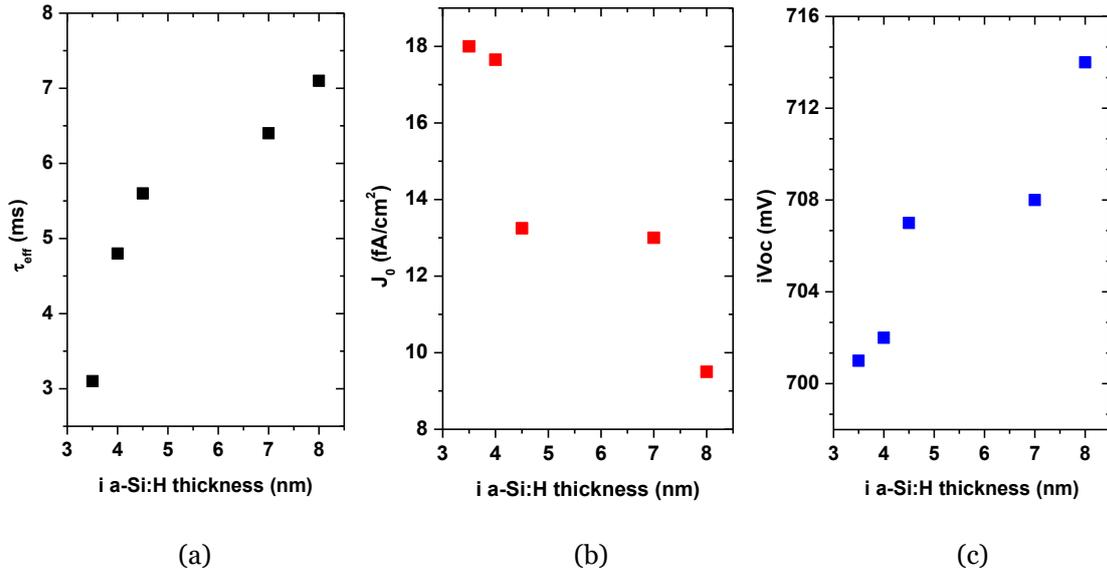
Figure 3.6: The effect of intrinsic a-Si:H thickness on: (a) minority carrier lifetime  $\tau_{eff}$  ( $\Delta=10^{15} \text{ cm}^{-3}$ ); (b) saturation current density  $J_0$  and (c)  $iV_{oc}$ . Measured on symmetric structures with a series of thickness of intrinsic a-Si:H: 3.5 nm, 4 nm, 4.5 nm, 7 nm and 8 nm, and fixed 6 nm n-type a-Si:H after 190 °C 30 min annealing on oven.
