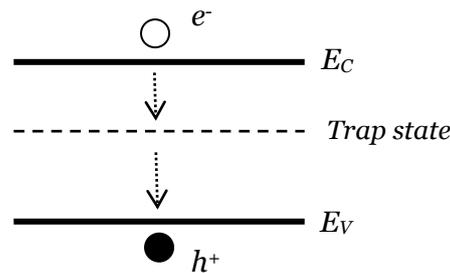
Figure 1.4: SRH recombination induced by trap state in the bulk.
