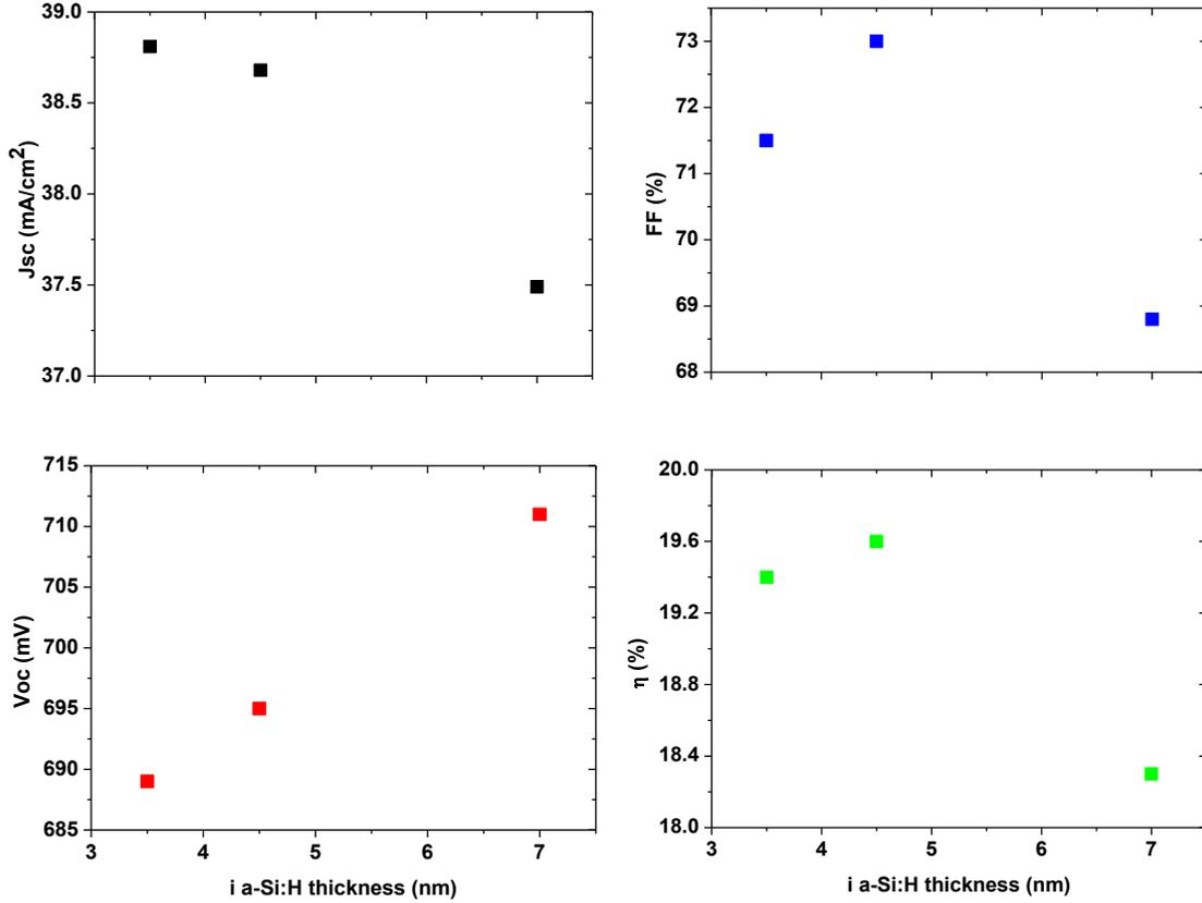
Figure 3.7: Characteristics of hybrid solar cells as a function of intrinsic a-Si:H thickness.
