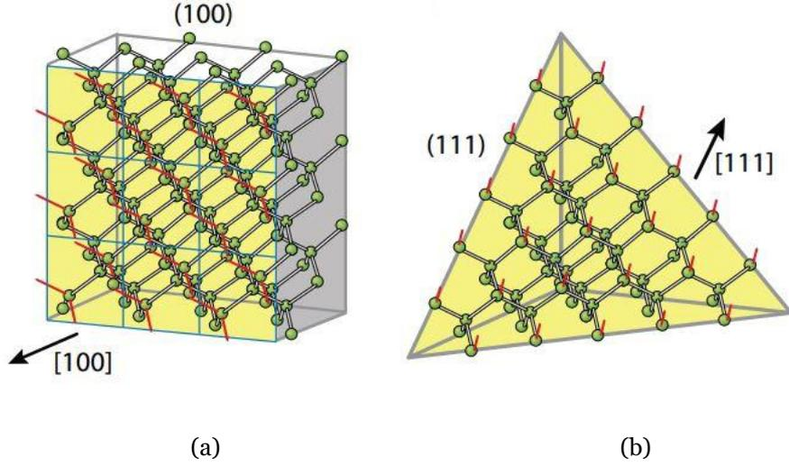
Figure 1.5: Lattice planes of (a) (100) surface, and (b) (111) surface in crystalline silicon [5]. The yellow planes are (100) and (111) surfaces respectively and the red lines stand for dangling bonds in the surface.
