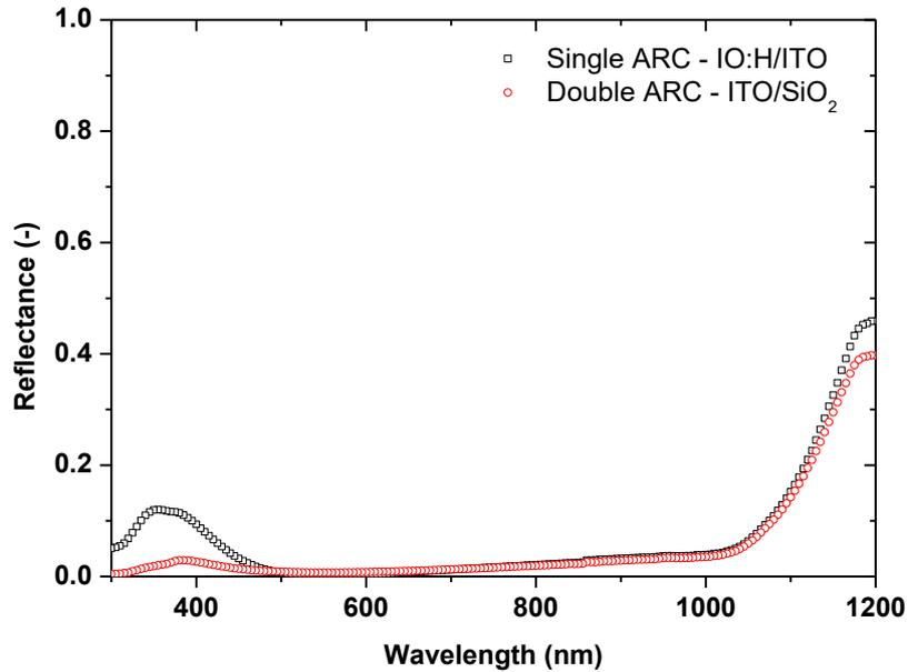
Figure 5.2: The measured reflectance spectra on textured wafers with single-layer ARC (65 nm IO:H/10 nm ITO) and double-layer ARC (40 nm ITO/90 nm SiO<sub>2</sub>).
