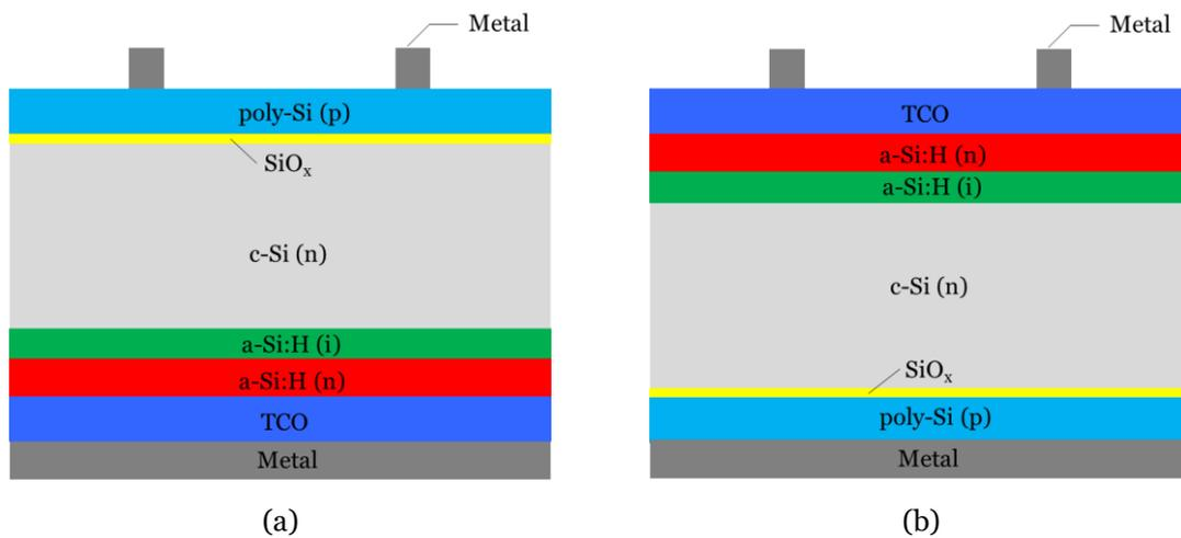
Figure 1.10: Possible structures of hybrid solar cells (not to scale): (a) n-type wafer with front emitter; (b) n-type wafer with rear emitter (priority in this thesis). Textured surface may be used to minimize external reflection and increase internal scattering for hybrid solar cells fabrication.
