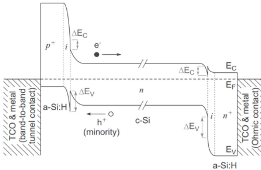
Figure 1.7: Schematic band diagram of SHJ solar cell [34].
