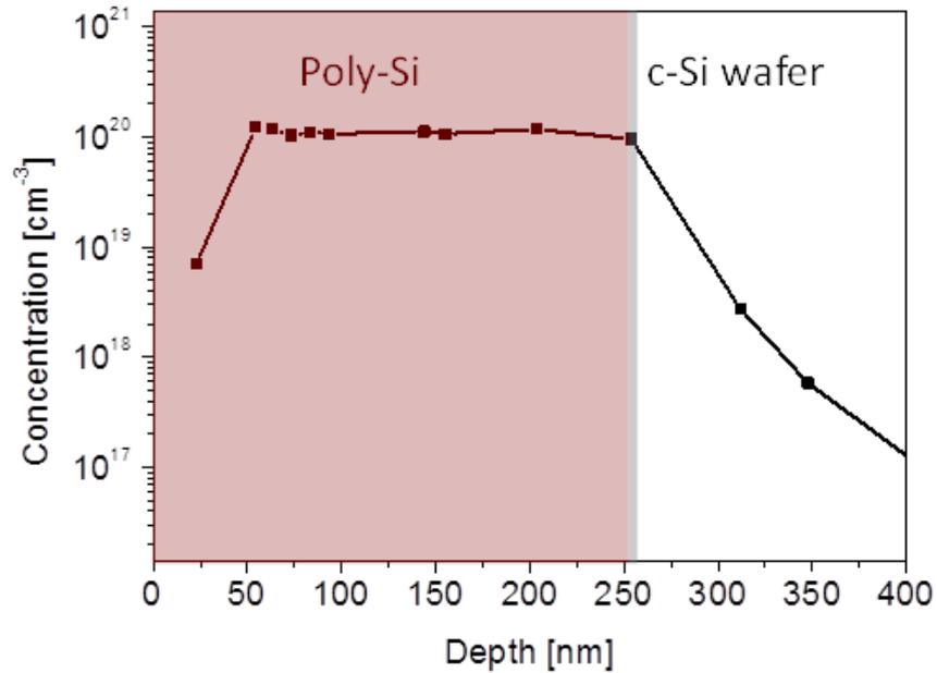
Figure 2.1: B-doping profile on 250 nm poly-Si passivating contacts (5 keV implantation energy, 5×10<sup>15</sup> ion/cm<sup>2</sup> dose and annealing at 950 °C in N<sub>2</sub>/O<sub>2</sub> atmosphere). Measured by ECV.
