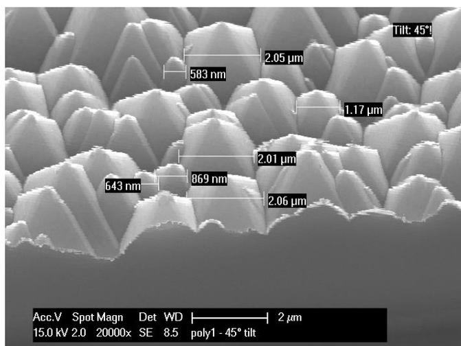
Figure 2.2: Front surface morphology after 20 min random pyramidal texturing in a solution of 5% TMAH with 120 mL ALKA-TEX. FREE. Taken in SEM.
