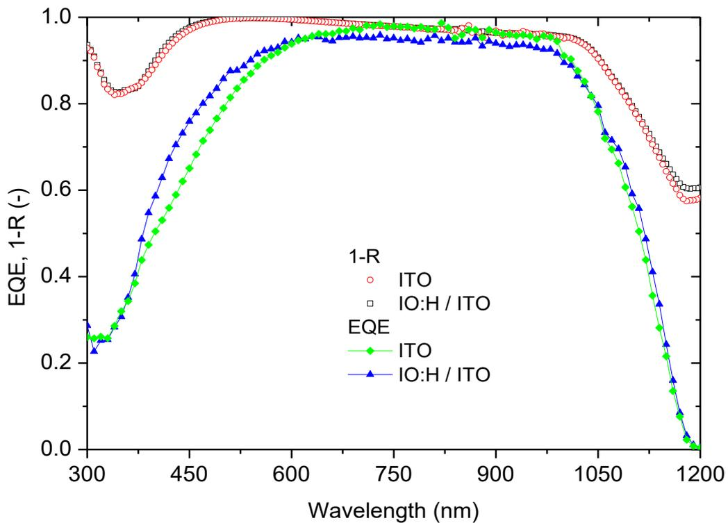
Figure 4.7: 1-R and EQE spectra of hybrid solar cells with two different TCO layers: ITO single layer with lower  $J_{sc}$  of  $38.64 \text{ mA/cm}^2$ ; IO:H/ITO stacks with slightly higher  $J_{sc}$  of  $38.96 \text{ mA/cm}^2$ .
