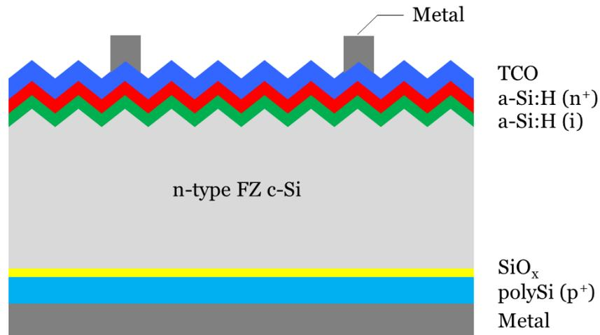
Figure 1.13: 2D schematic structure of hybrid solar cells (not to scale).
