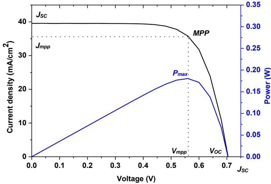
Figure 2.8: Illuminated J-V curve (black) and power output (blue) of  $9 \text{ cm}^2$  hybrid solar cell under AM 1.5 illumination.
