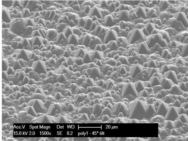
Figure 1.12: Wafer surface morphology after 30 min random pyramidal texturing in a solution of 5% TMAH and 5 mL ALKA-TEX. FREE. Taken in SEM.
