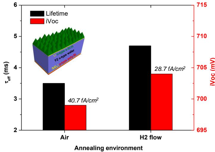
Figure 3.8: Lifetime ( $\Delta=10^{15} \text{ cm}^{-3}$ ),  $iV_{oc}$  and  $J_0$  measurements on precursor cells (3.5/6 nm i/n stacks as FSF) in ambient air and  $H_2$  annealing environment. Air annealing condition is 190 °C ambient air for 30 min on oven and  $H_2$  annealing is 200 sccm  $H_2$  flow for 30 min on 180 °C Amor chamber.
