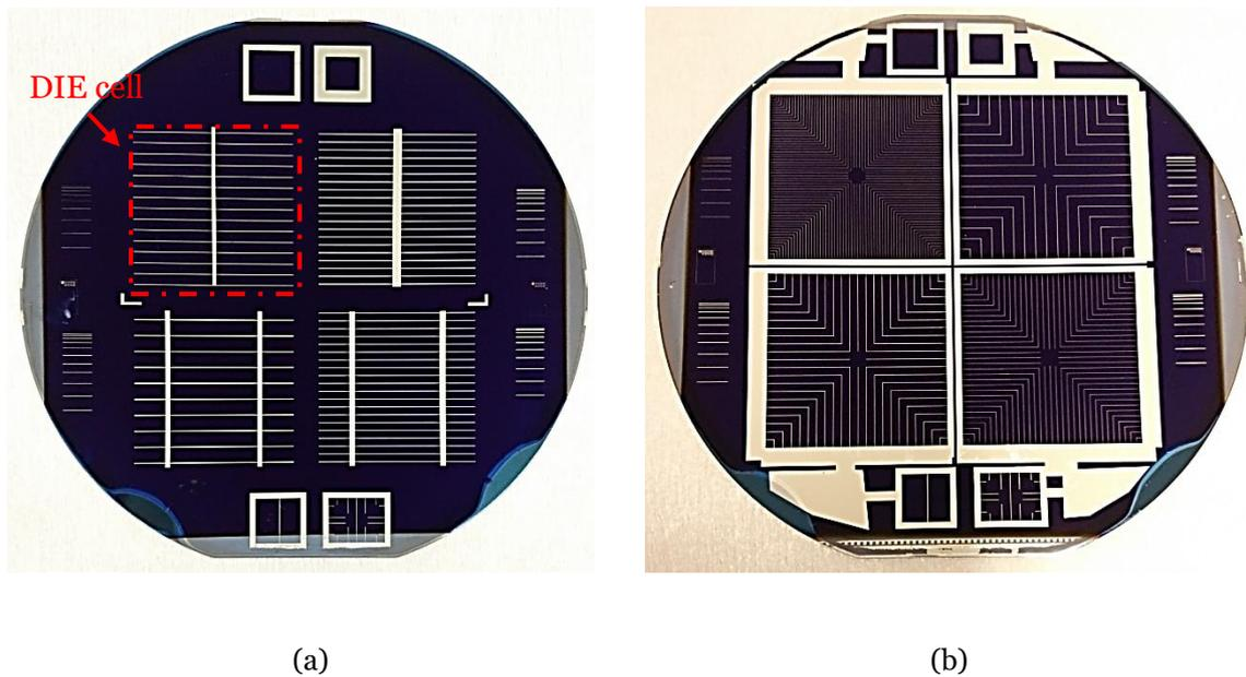
Figure 2.4: Pictures of hybrid solar cells with two different metal patterns fabricated in the facility of PVMD group at Delft University of Technology. A wafer consists of four DIE cells in the middle. (a) 2.8 cm × 2.8 cm DIE cell with busbars in the middle; (b) 3 cm × 3 cm DIE cell with busbar at the edge.
