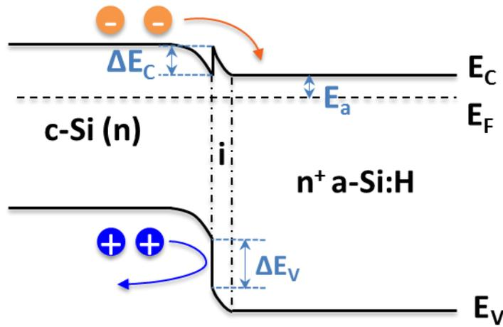
Figure 3.1: Schematic band diagram of a-Si:H (n)/a-Si:H (i)/c-Si (n) structure.
