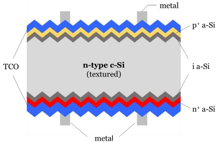
Figure 1.6: A schematic structure of n-type SHJ solar cell.
