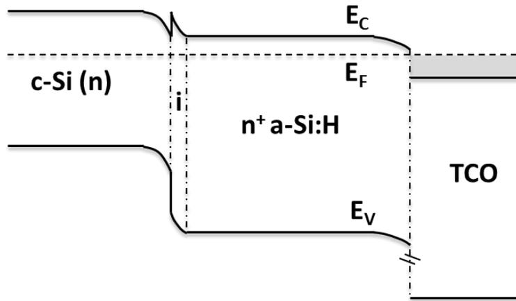
Figure 5.1: Schematic band diagram of  $c\text{-Si}(n)/a\text{-Si:H}(i/n)/\text{TCO}$  structure with  $W_{TCO}$  lower than  $n$ -type  $a\text{-Si:H}$ .
