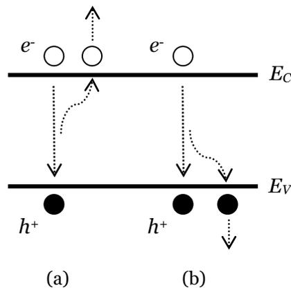
Figure 1.3 : Auger recombination in the bulk: (a) eeh interaction and (b) ehh interaction.
