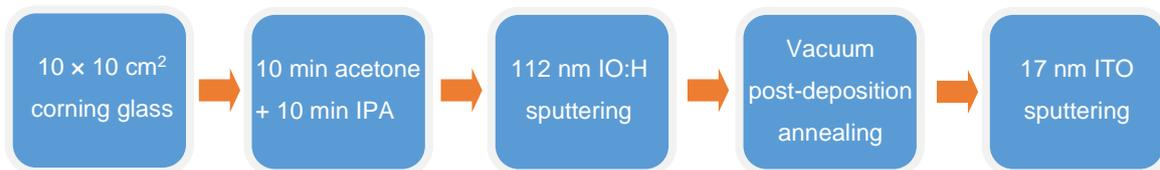
Figure 4.3: Flowchart of glass samples with 129 nm IO:H/ITO stacks. The ratio of the IO:H (20 W)/IO:H (135 W)/ITO (200 W) layers thickness is 1 : 5.5 : 1, the same ratio as on the textured surface.
