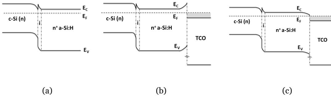
Figure 4.1: Schematic band diagram illustrating the effect of TCO work function on band alignment at a-Si:H (n/i)/c-Si (n) structure: (a) without TCO; (b) TCO work function higher than a-Si:H (n); (c) TCO work function lower than a-Si:H (n).
