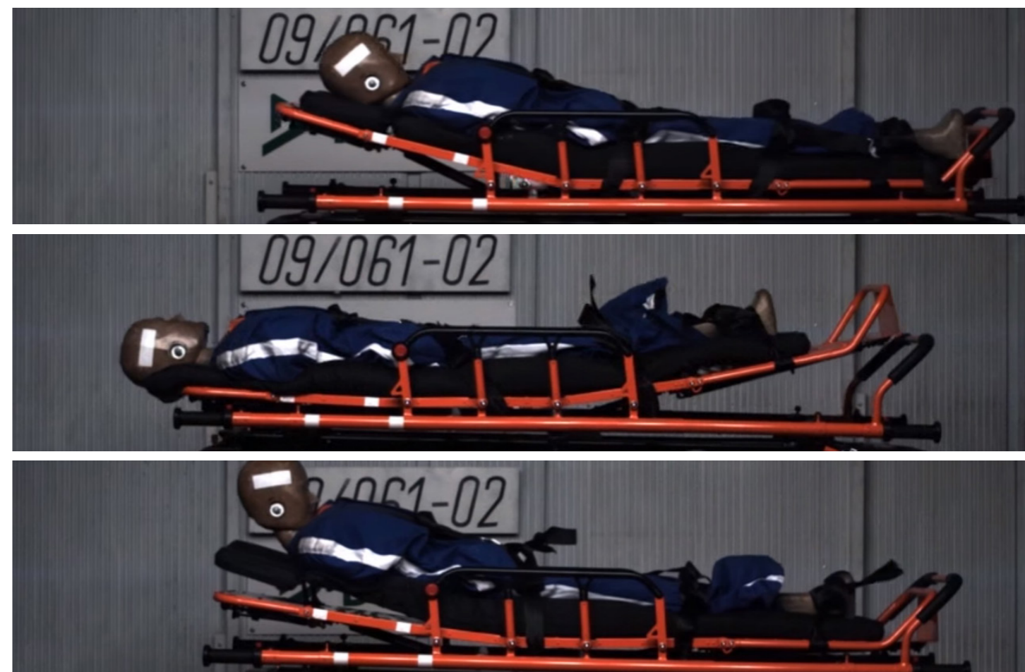
Figure 5.9 Crash test picture sequence using inversed crash sled. Snapshots required from Youtube. Acquiring footage from visit to Tass International was not possible due to non-disclosure agreements.
