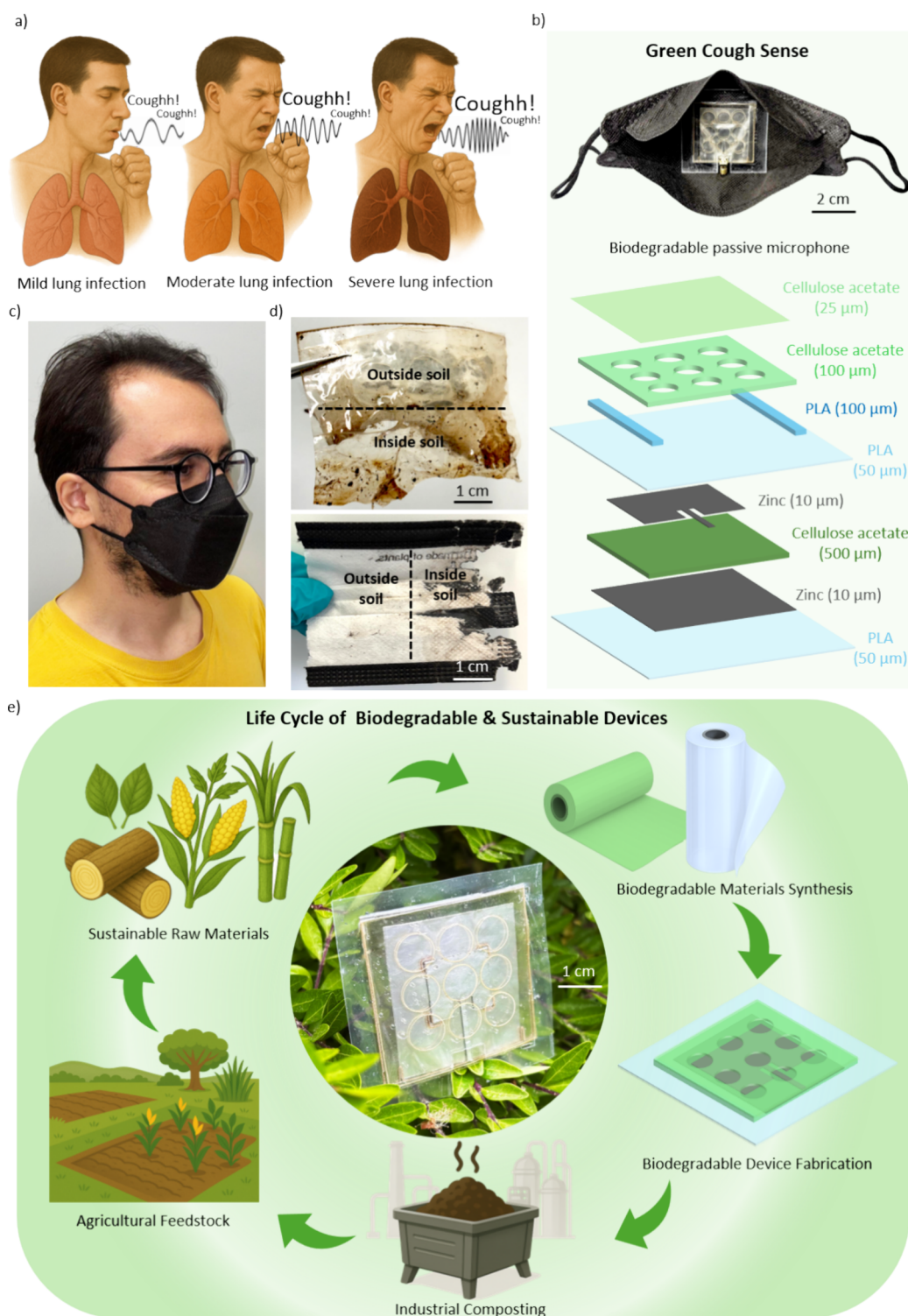
Figure 1. Green Cough Sense is an eco-friendly smart face mask that monitors respiratory health by analyzing cough acoustic signals: passive, battery-free, and entirely biodegradable, with zero electronic waste and manufactured using low-temperature, green processes. (a) The severity of respiratory complications can be assessed by analyzing cough sound dynamics, including intensity, duration, rate, and frequency components. (b) The system features a biodegradable polylactic acid (PLA) face mask housing a passive microphone, which integrates an array of drum-like membranes that vibrate in response to sound waves. These vibrations alter the near-field of an integrated patch antenna, modulating its electromagnetic scattering parameters. (c) Photographs of the wearable device, shown before and after partial degradation in soil. The microphone consists of a 3D vertical stack of laser-patterned layers made from cellulose acetate (CA), PLA, and zinc, bonded through a low-temperature lamination process. (d) Image of the partially degraded microphone and face mask after soil burial under industrial composting conditions. (e) Schematic of the device life cycle—from sourcing sustainable raw materials (including soil enriched by previously composted devices), through cleanroom-free green fabrication, to end-of-life biodegradation, returning safely to the environment as nutrient-rich soil. The male model imagery is partially AI-generated. In panel (e), the inset images of industrial composting, agricultural feedstock, and sustainable raw materials contain AI-generated elements.
