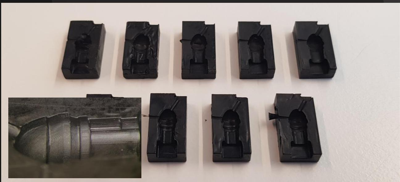
Figure 82: Powder Injection Moulding test pieces; each row from one mould, moulded from left to right
