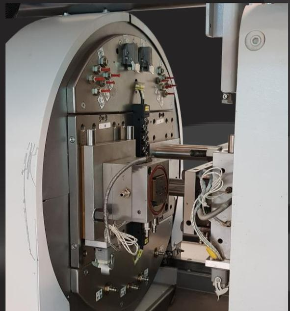
Figure 14: Master mould inside injection machine
