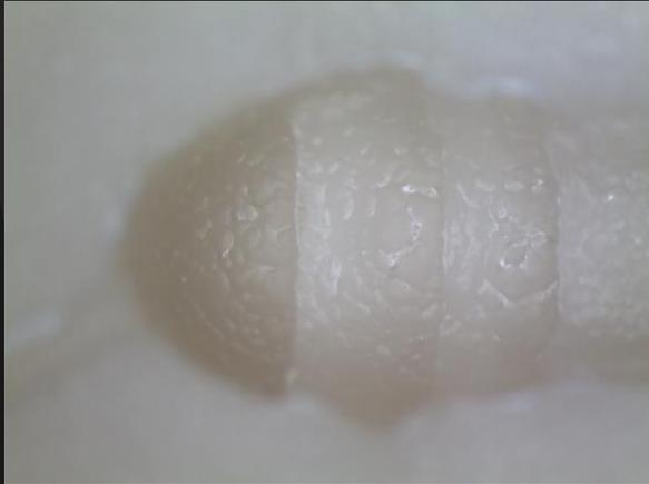
Figure 78: Bubble pattern ceramic mould surface
