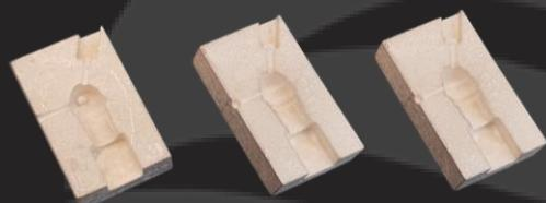
Figure 67: Casted mould halves with researched investment
