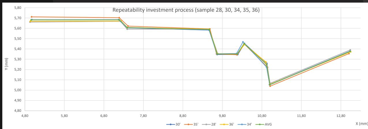
Figure 62: Measured point of the sintered cast to test the repeatability of the method
