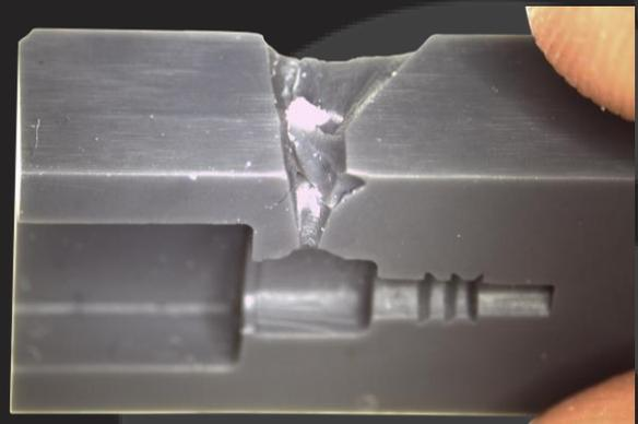
Figure 17: Mould wear
