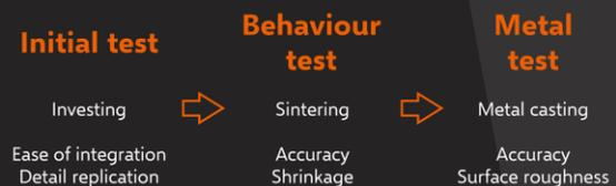
Figure 61: Test procedure micro casting
