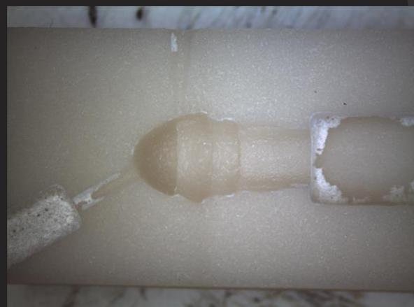
Figure 77: Ceramic part made with pressing investment
