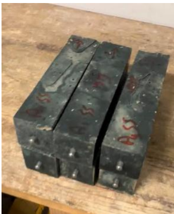
Figure 3.5: Dry shrinkage setup.
