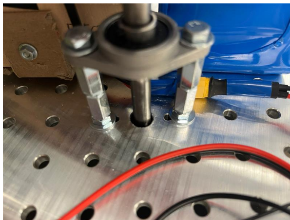
Figure 8.1: Misaligned central rod and bearing structure
