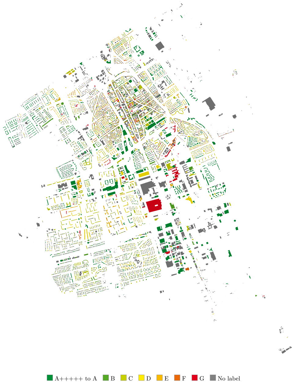
Figure 6.9: Delft, shown as building footprints coloured by the average EP-Online energy label of the addressable units ( verblijfsobjecten ) they contain. North-oriented top view. Screenshot of KITModelViewer (KIT); model by the author.
