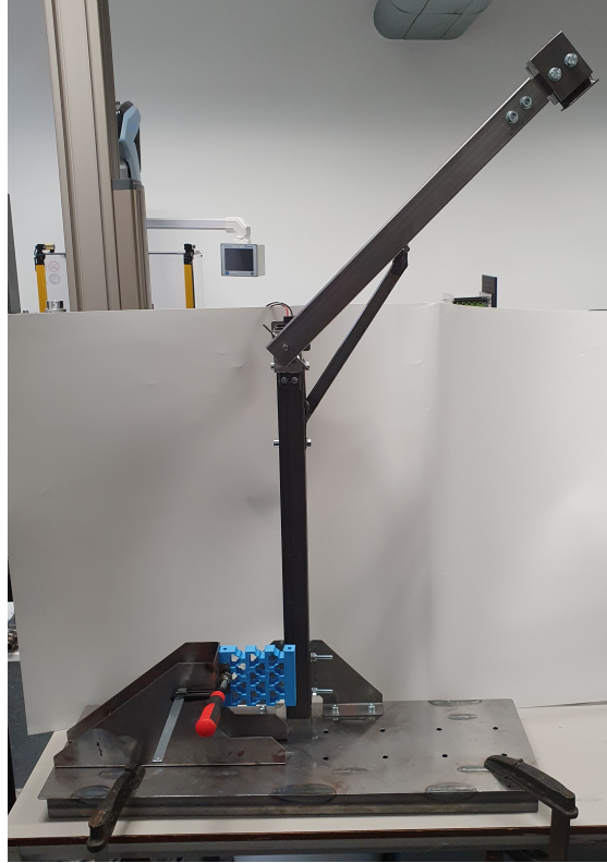
Figure 3.7: Pictured is the dynamic tester with a sample mounted and ready for testing. Table clamps were used to prevent the tester from moving due to the impact force.
