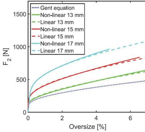
**Figure 6: Difference between the linear (solid line) and non-linear (dashed line) material model for a range of thicknesses. Results for the linear model correspond to  $E = 12.25$  MPa. The used mesh is shown in Figure 5.**
