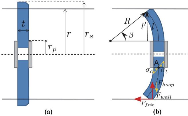
**Figure 2: (a) Sketch of an undeformed sealing disk at rest. (b) Sketch of a sealing disk moving inside a pipe.**
