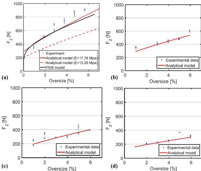
**Figure 7: (a-d) Comparison of the analytical model with experimental results. Properties of disk are summarized in Table 1. The letter assigned to each disk in Table 1 corresponds to the letter of the panels in this figure.**
