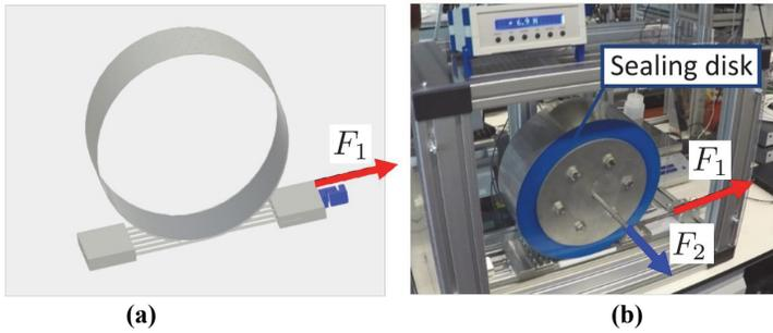
**Figure 3: (a) Schematic of the setup. (b) Photograph of the experimental setup with a sealing disk.**
