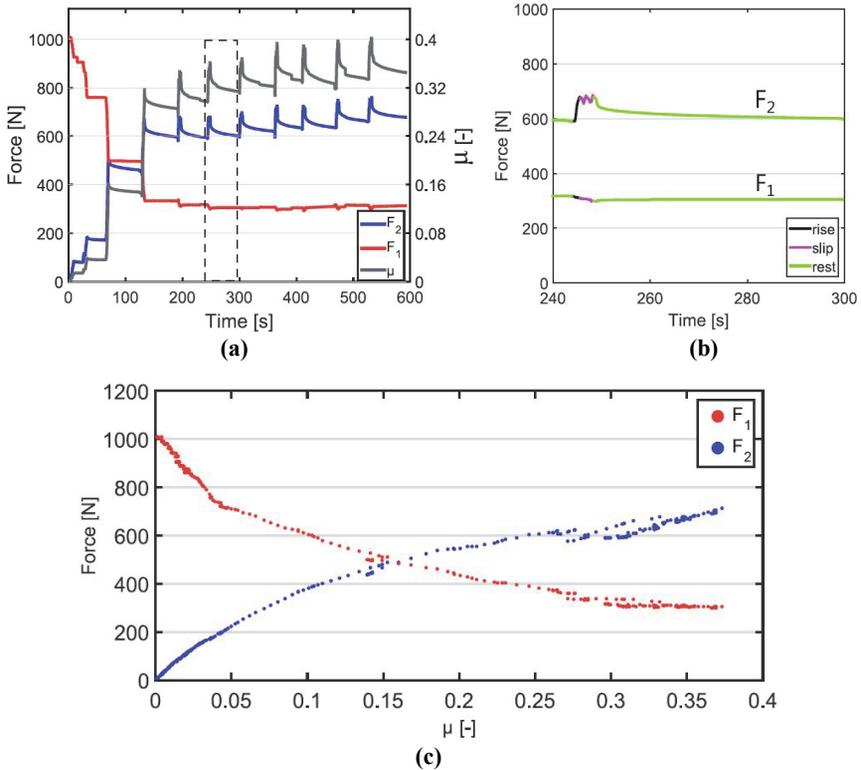
**Figure 4: (a) Time series of  $F_1$  and  $F_2$  and the corresponding value for  $\mu$ . (b) A close up of  $F_1$  and  $F_2$  between 240 and 300 seconds, which is indicated in panel a with the dashed box. (c)  $F_1$  and  $F_2$  plotted for different values  $\mu$ , including only the points that have been recorded during the rise zone.**
