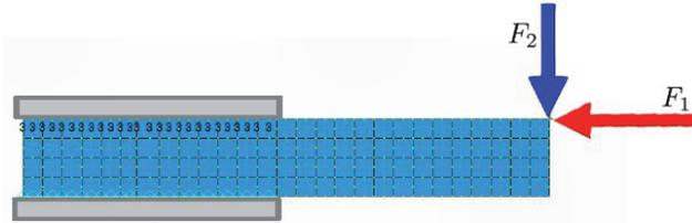
**Figure 5: Finite element mesh of a sealing disk in axisymmetric perspective. The two forces  $F_1$  and  $F_2$  are applied as shown. By fixing the ratio between  $F_2$  and  $F_1$  the coefficient of friction  $\mu$  is imposed.**
