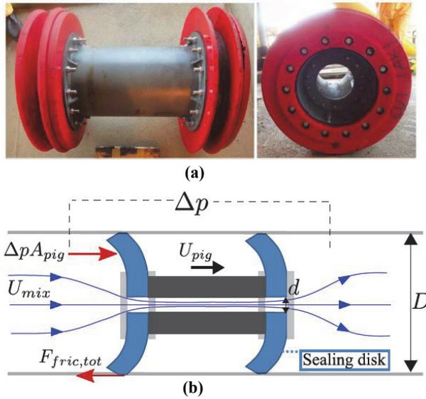
**Figure 1: (a) Example of a by-pass pig. Reproduced from [12]. (b) Schematic representation of the force balance on a by-pass pig.**
