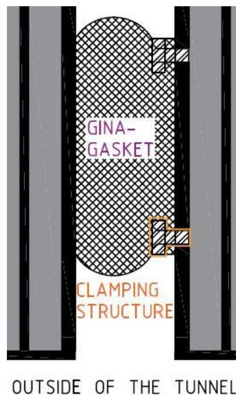
Figure 18: Cross section of the Gina-seal, showing the outside of the tunnel, and the difference between the clamping structure and the Gina-gasket
