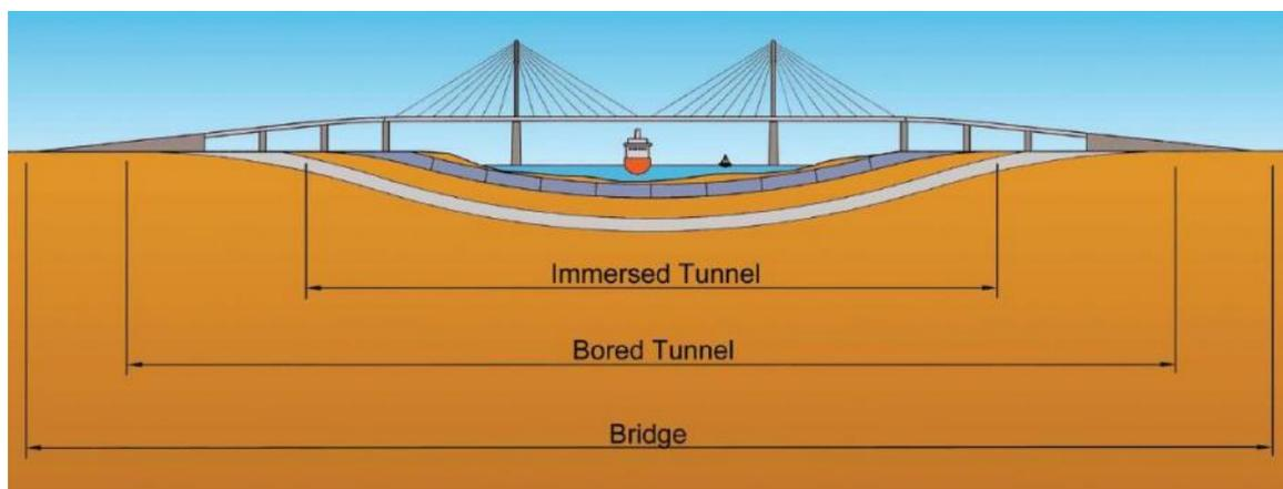
Figure 1: Depth and length of an Immersed tunnel compared to a bored tunnel and a bridge (ITA, 2011)
