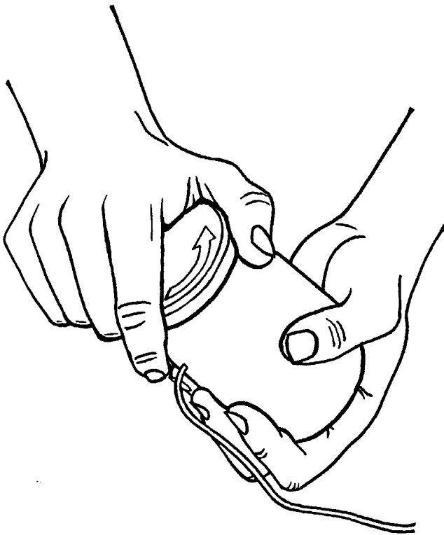
Figure 2.3.1 The handling of the jam-jar-shaped force meter, the subject was to choose how to hold the handle in his hands. (Figure by J. Trappenburg)
