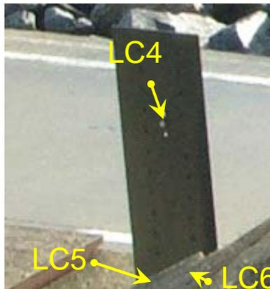
**Fig. 73:** Load cells installed at the large dummy D2
