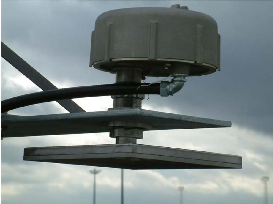
**Fig. 8:** *Installed Wave Guide Radar at the measurement site*
