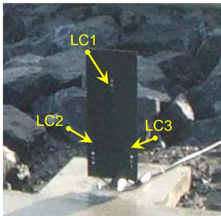
**Fig. 71:** *Load cells installed at the little dummy*
