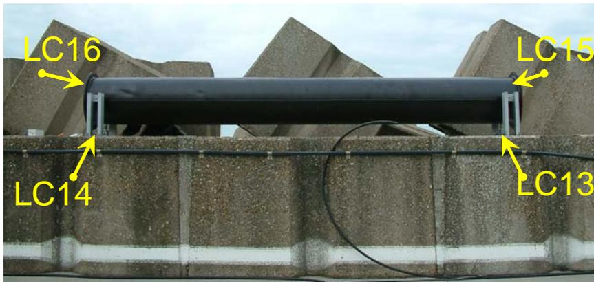
**Fig. 77:** Load cells installed at the pipeline
