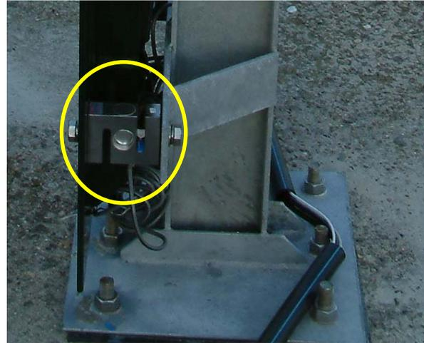
**Fig. 28:** *Detail of mounted load cell*
