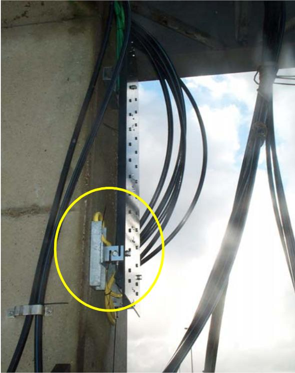
**Fig. 34:** Measurements of forces on a vertical wall: detail with the circle indicating mounted S-shaped load cell
