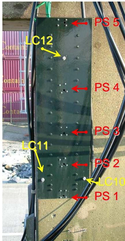
**Fig. 80:** Load cells(LC) and pressure sensors (PS) installed at the vertical wall
