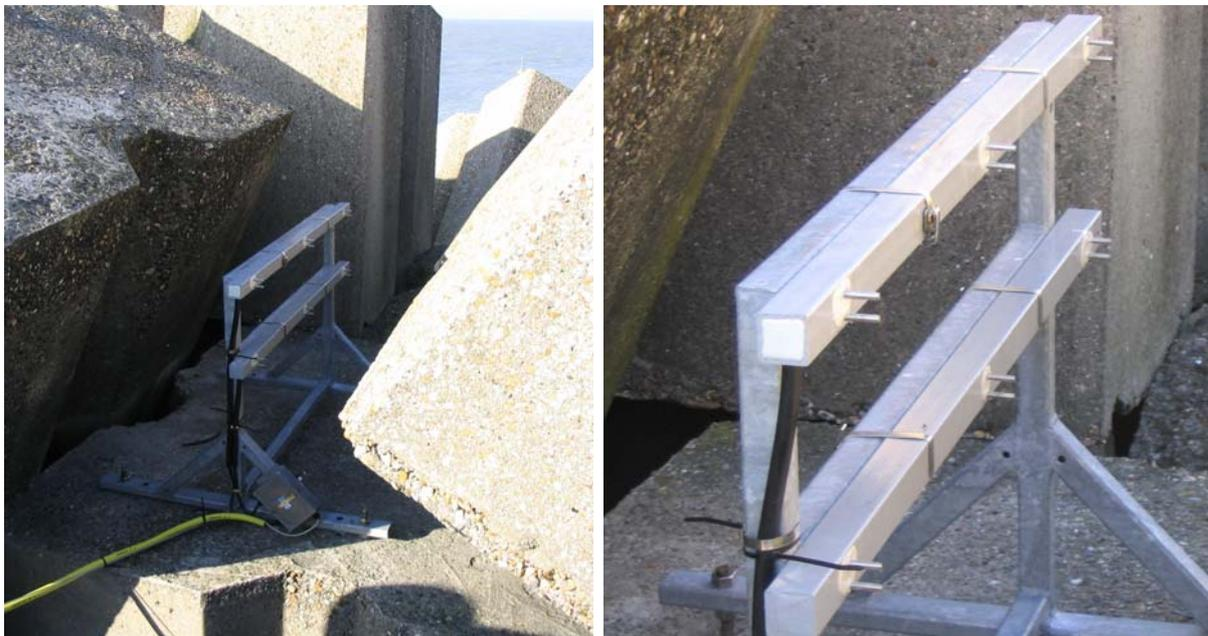
**Fig. 37:** *Velocity meter in front of the pipeline*
