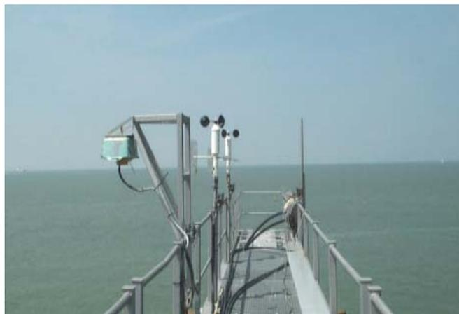
**Fig. 9:** *Infra-red wave height meter and combined wind sensor at the measurement jetty*
