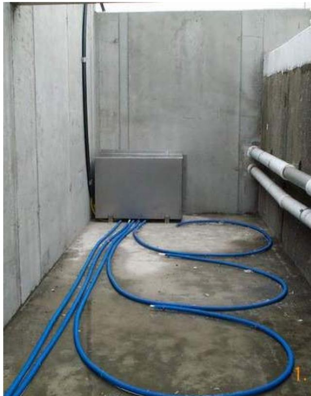
**Fig. 17:** *Five tubes placed at the bottom of the tank allow to measure the pressure at five different places*
