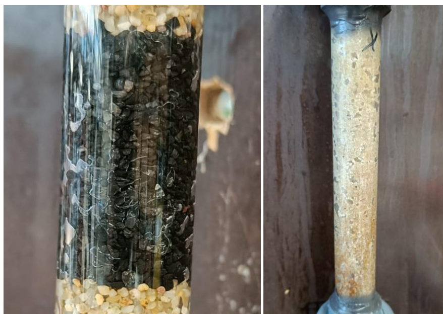
Figure 16A-B Air entrapment in (A) column 1 (GAC-N) and (B) column 2 (SSF) observed during week 5.5
