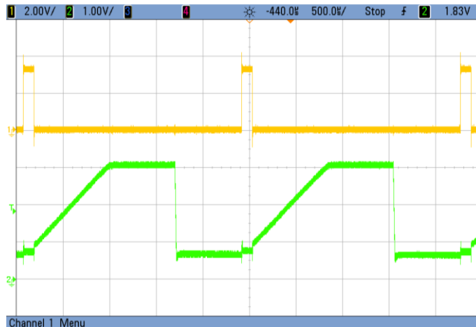
Figure 7-14. The measure output waveform of CTIA pixel.
