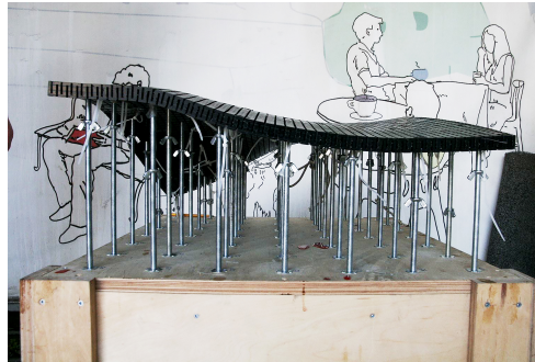
Figure 1 FlexiMold Flexible Formwork Device.
