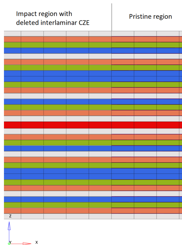
Figure 5.46: Modelling approach of impact damage as multiple delaminations in FE model.
