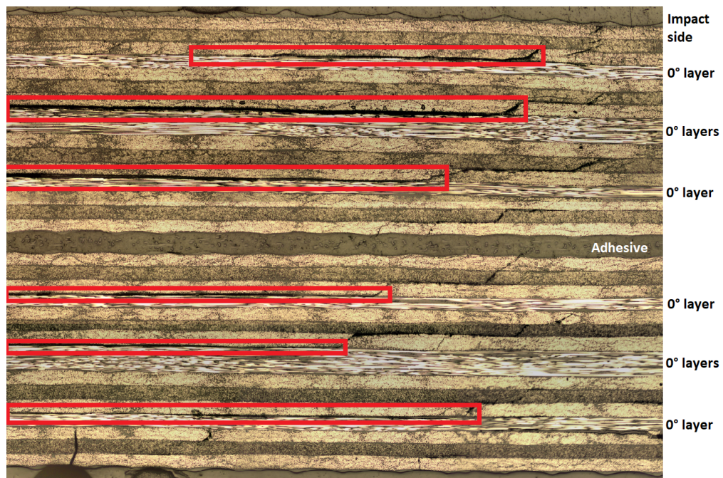
Figure 5.43: Delamination pattern in SLTAI30 specimen after impact with 10J energy.
