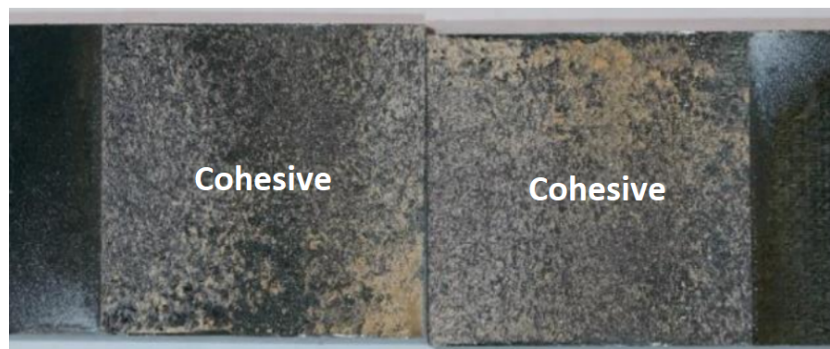
Figure 5.13: Experimental failure mode of SLS0.
