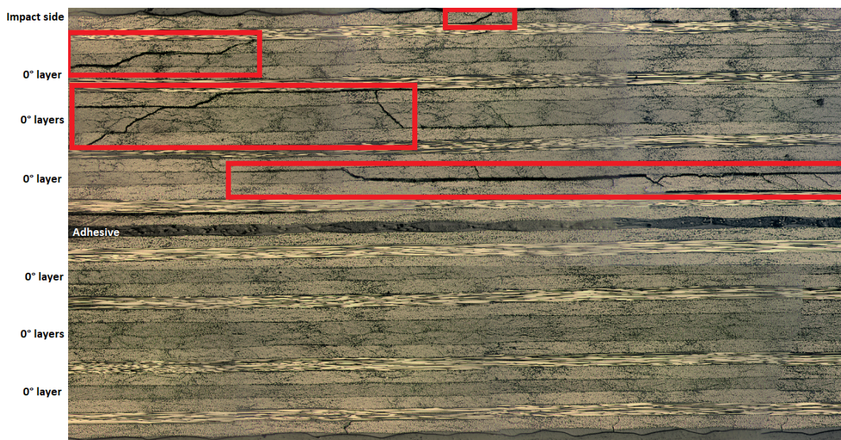
Figure 5.41: Damage in SLTAI30 after impact with 15J energy.
