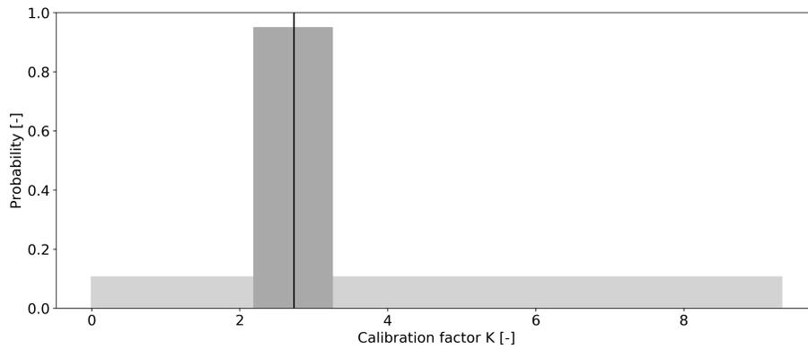
Figure 8: Probability density distribution of model calibration factor  $K$ , prior to the GLUE calibration procedure (light grey) and posterior (dark grey). The black line indicates  $K = 2.73$ , the value with the highest  $NS$  skill score.
