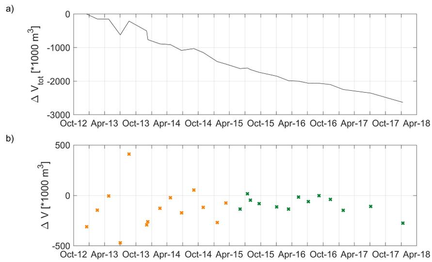
Figure 3: Total volume change ( $\Delta V_{tot}$ ) since December 2012 (a) and volume change ( $\Delta V$ ) between consecutive surveys (b) of the central, net eroding area of the Sand Engine. Orange crosses are used for model calibration and green crosses are used for validation. The positive volume change in August 2013 is influence by measurement errors.
