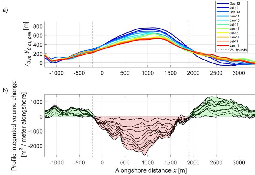
Figure 2: Morphological evolution of the Sand Engine since December 2012. Coastline position,  $y_{0m}$ , with respect to a reference coastline,  $y_{0m,pre}$ , prior to construction of the nourishment (a) and profile integrated volume change since December 2012 (b). The green shaded areas denote net sedimentation and the red shaded area denotes net erosion.
