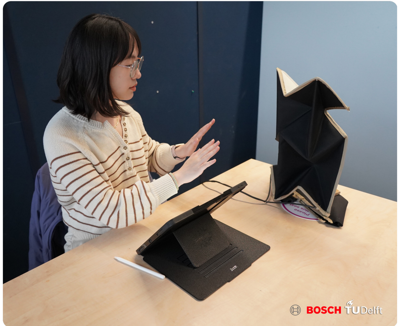
Figure 39: 160-watt radiant foldable-panel heater provides space-saving warmth.
