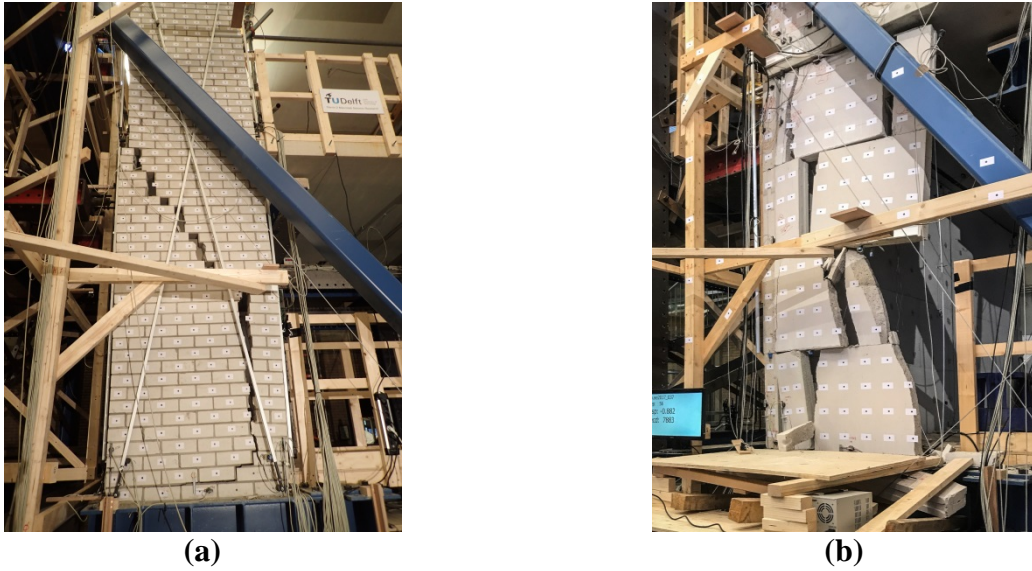
Figure 5: Main damage in the wide piers at the ground floor: (a) CS brick masonry assemblage ( d_2 = 82 mm); (b) CS element masonry assemblage ( d_2 = 54 mm).
