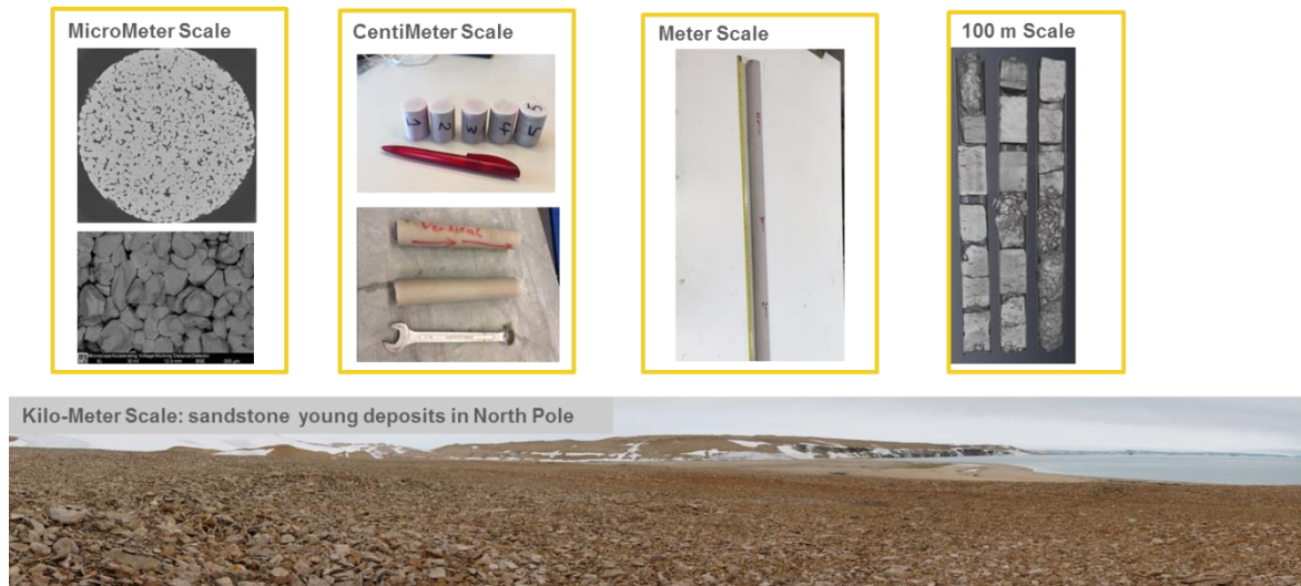
Figure 1.6: Scale-window of sandstone from micrometre scale to kilometre scale. Microeter scale → SEM and micro CTS, CentiMeter Scale → Plugs and cores, Meter Scale → One meter core at 3.9 cm diameter, Kilo-Meter Scale → Artic glacier landscapes with moraines from fines to pebble size compositions, location in Svalbard archipelago, Nordauslandet – Vibebukta.
