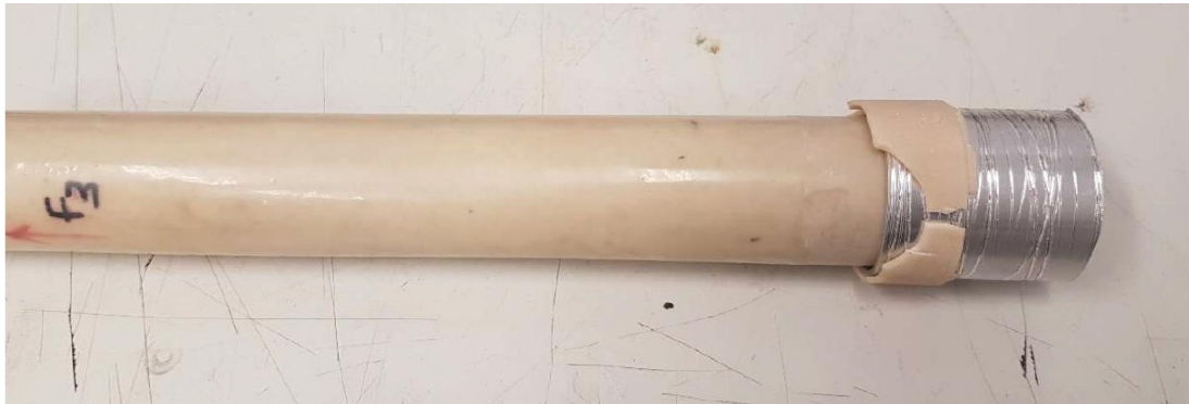
Figure App1: Core to be stacked with guiding aluminium tube.
