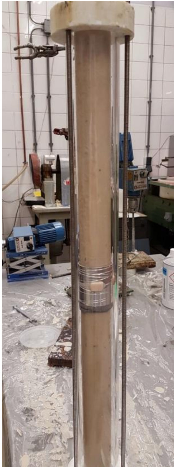
Figure App2: Stacked cores before being cast in glue
