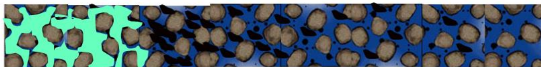
5- Oil ganglia coalesce further and become more stabilized. Water is flowing out of the porous media, influencing/causing some oil movement at the front of the oil bank
