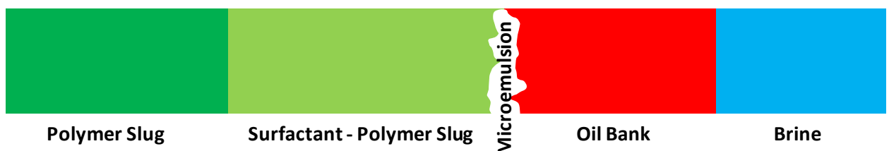
Figure 4.15 represents a schematic of the slug sequence in the porous media. The microemulsion phase appears in the front of the chemical slug and the tail of the oil bank. Literature showed that the viscosity of micro-emulsions at optimal salinity is greater than the oil viscosity (SPE 179672).
