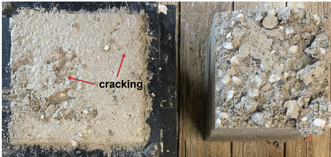
Figure 4.2: Cracking and swelling of AAC containing untreated MSWI BA aggregates after 1-day (100% replacement of gravel (4-8 mm))
