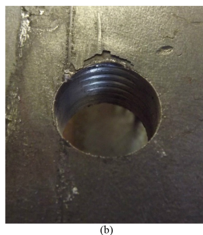
Fig. 12. Observed damages (P3.1-1) (a) bearing deformation and (b) thread penetration in the steel beam.
