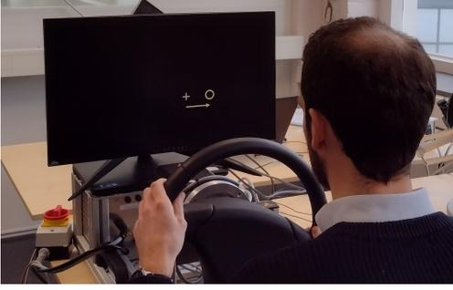
(a) The experiment consisted of a steering task, in which both the participant and the control algorithm were tasked with compensatory tracking of the yellow circle, controlling the grey plus.
