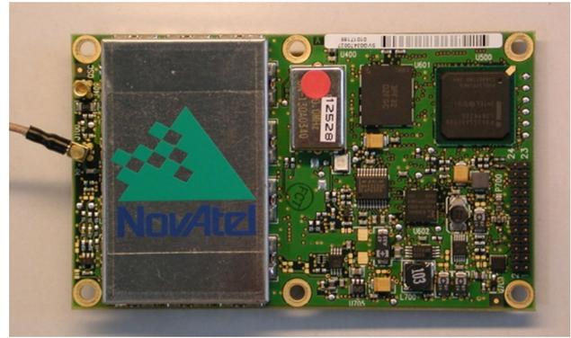
**Fig. 2** NovAtel OEM4-G2L GPS receiver. Image DLR
