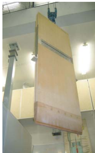
Figure 4. The windtunnel model; cavity with embedded splitter plate.
