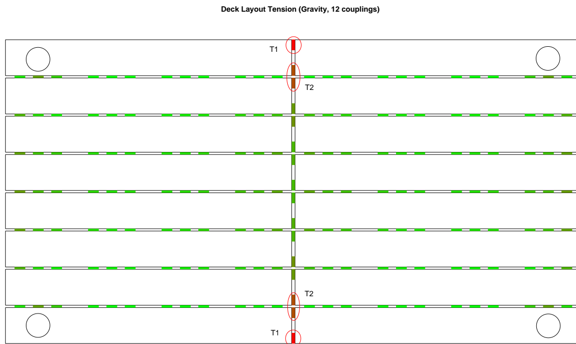
Figure 5.6: Colour visualisation of tensional loading for gravity case (12 couplings)
