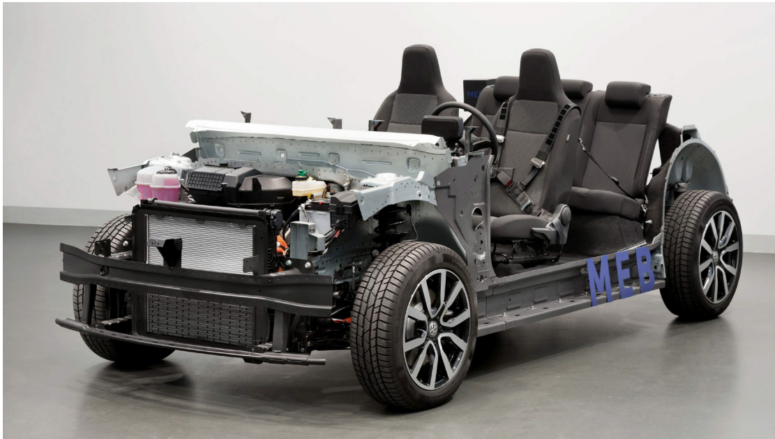
image / figure 1: The Volkswagen MEB-platform is an example of how platforms are used in the automotive industry
