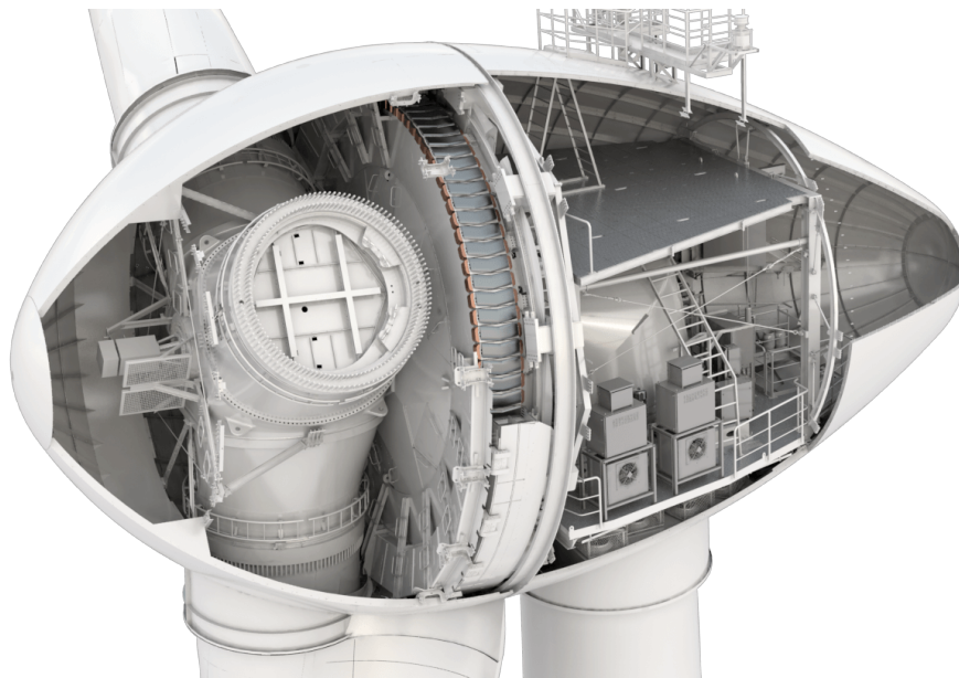
Figure 5.2: Enercon E-126 nacelle
