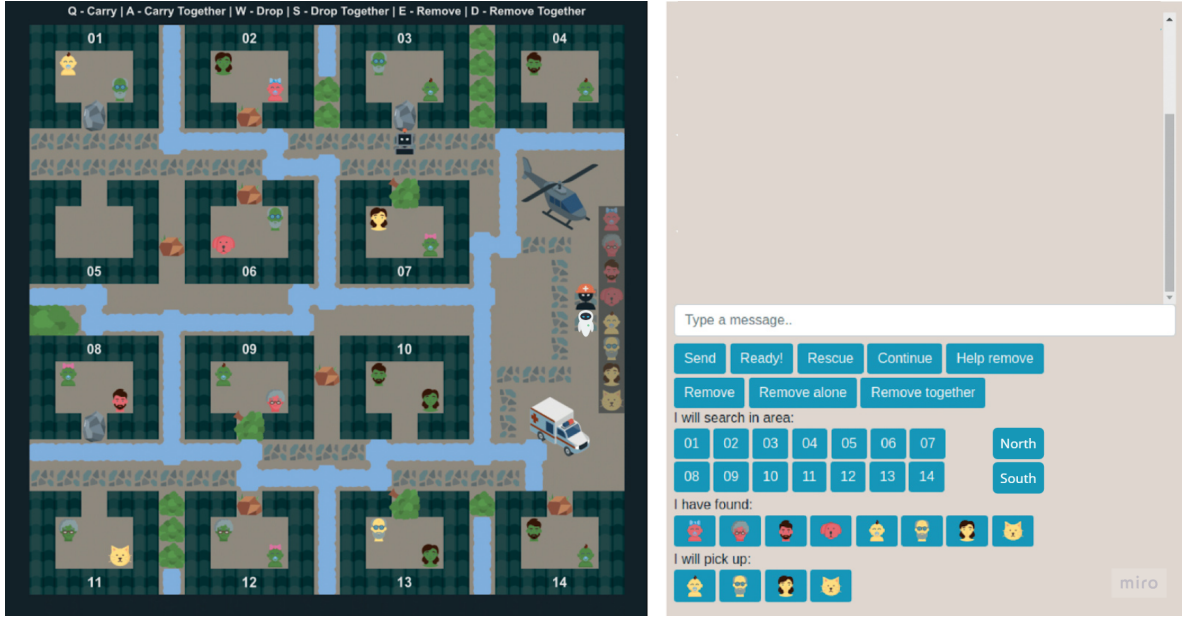
Figure 3.2: The simulated search and rescue environment built using MATRX. Fourteen houses containing victims and three rescuers to save the injured in a top down view on the left. Communication buttons and chat box on the right.
